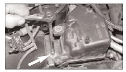
MAP sensor electrical connection from the stock intake tube as shown.
