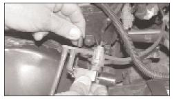
16. Using the provided rubber cap, plug the port on the solenoid from step 15 as shown. (VTEC only)
