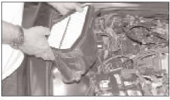
10. Pull upwards to remove the lower air cleaner assembly as shown.
