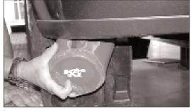
42. From underneath the vehicle install the K&N<sup>®</sup> air filter onto the cold air tube and secure with the provided hose clamp.
