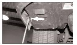
19. Raise the vehicle and support it with jack stands then remove the bolt on the lower valance as shown.
