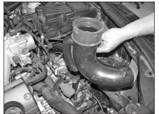
23. Remove the air inlet duct as shown.
