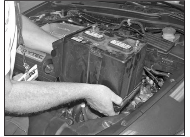
19. Remove the battery and the plastic cover as shown.
