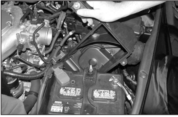
10. Pull up to release the lower air cleaner assembly from the stock air inlet duct and remove as shown.
