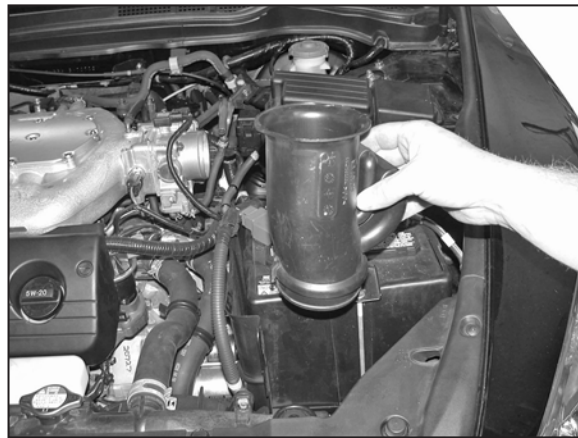
16. Remove the air inlet duct as shown.
