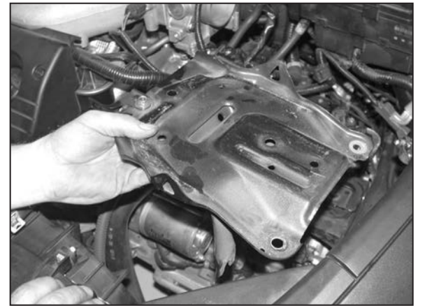
21. Remove the battery tray as shown.
