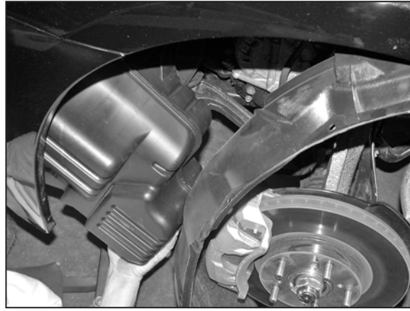
14. Remove the air intake resonator as shown. NOTE: Not all air intake resonators may look the same.
