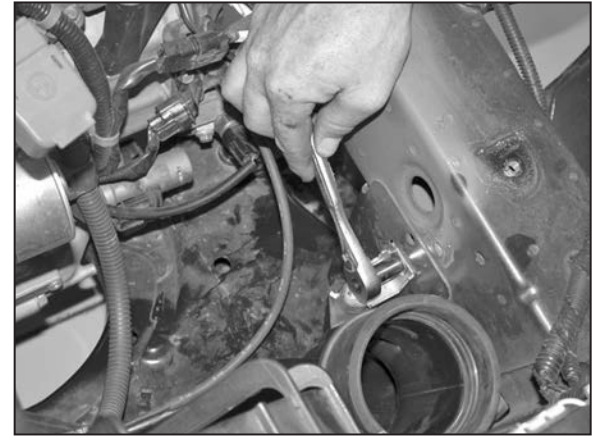
22. Loosen and remove the bolt that secures the air inlet duct to the inner fender as shown.
