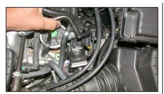
4. Disconnect the crankcase vent hose from the stock intake tube as shown.
