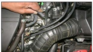
3. Disconnect the vent from the stock intake tube as shown.
