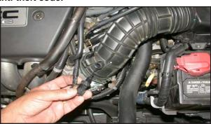
2. Remove the air temperature sensor from the stock intake tube as shown.
