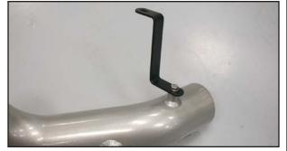
17. Install the "Z" bracket onto the K&N® short ram tube using the provided hardware as shown.
