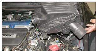
8. Remove the complete air cleaner assembly as shown.
