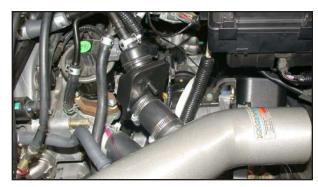
24. Install the crankcase vent chamber onto the vent on the K&N® short ram tube, then, connect the other end to the crankcase vent hard line as shown
