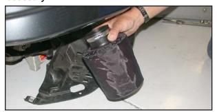
31. Install the air filter from underneath the vehicle and secure it with the provided hose clamp as shown. Tighten hose clamp from step 28.
