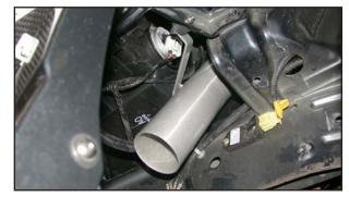
29. Line up the tube bracket with the rubber mounted stud and secure with the provided hardware as shown.
