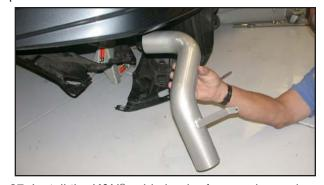
27. Install the  $K\&N^{\tiny \circledcirc}$  cold air tube from underneath the vehicle as shown.
