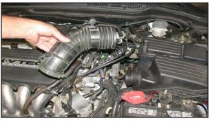
5. Loosen the hose clamp at the throttle body and remove the stock intake tube as shown.
