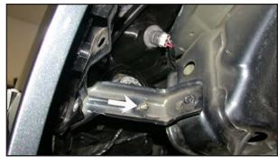
26. Install the provided rubber mounted stud onto the front of the fender brace and secure with the provided hardware as shown.
