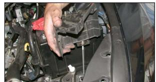
9. Remove the air inlet cover, which is secured to the radiator core support by two plastic rivets.
