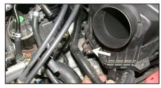
7. Unclip the wire harness from the bottom of the air cleaner assembly as shown.
