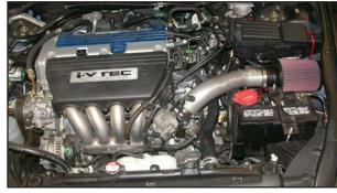
35. This K&N® high flow intake system has been designed to be used in two different configurations. In the case of inclement weather, the cold air tube can be removed and the air filter can be clamped onto the intake tube located in the engine compartment to avoid the possibility of ingesting water into the engine.
