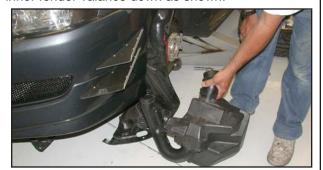
13. Remove the two bolts that secure the resonator to the inner fender, then, remove the resonator at shown
