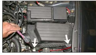
6. Loosen the two air cleaner bolts as shown.
