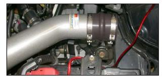
25. Install the silicone hump hose and hose clamps onto the  $K\&N^{@}$  short ram tube as shown.
