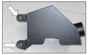
12. Install the mounting grommets from the previous step into the heat shield as shown.
