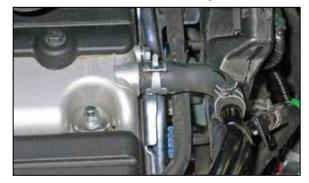
9. Release the spring clamp securing the crank case vent hose to the valve cover and then disconnect the hose from the valve cover.
