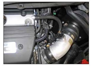
27. Install the provided silicone hose onto the  $90^{\circ}$  fitting attached to the K&N<sup>®</sup> intake tube. Attach the open end of the hose to the valve cover port as shown.
