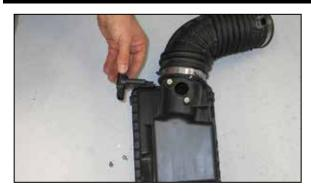
24. Remove the two screws securing the mass air sensor into the factory air box, then remove the sensor from the air box.
