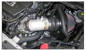
26. Install the K&N<sup>®</sup> intake tube assembly into the silicone hump hose and then into the throttle body's silicone hose. Align the tube and then secure with the provided hose clamps.
