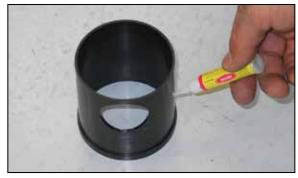
21. Apply several drops of the provided "Super Glue" to the lip of the venturi as shown.
