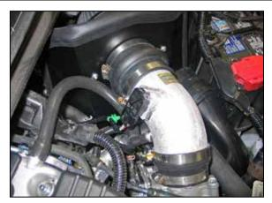
28. Reconnect the mass air sensor electrical connection.
