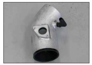
23. Install the provided 90° vent fitting into the K&N<sup>®</sup> intake tube as shown. NOTE: Plastic NPT fittings are easy to cross thread. Install the vent fitting "hand" tight, then turn it two complete turns with a wrench.
