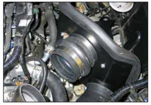
19. Install the provided silicone hose (5-576) onto the filter adapter and secure with the provided hose clamp.
