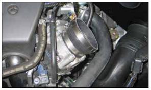
18. Install the provided silicone hose (084034) onto the throttle body and secure with the provided hose clamp.
