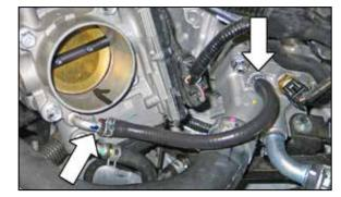
10. Be sure the engine is cool, then disconnect the coolant by-pass hoses from the engine and intake manifold. Install the provided coolant by-pass hose and secure with the factory spring clamps.
