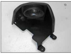
14. Install the filter adapter into the heat shield and secure with the provided hardware.
