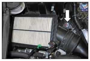
6. Remove the lower air box retaining bolt shown.
