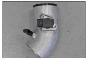
25. Install the mass air sensor into the K&N<sup>®</sup> intake tube and secure with the provided hardware.
