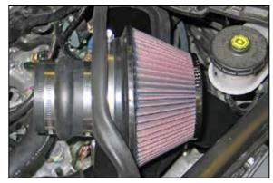
20. Install the K&N® air filter and secure with the provided hose clamp.
