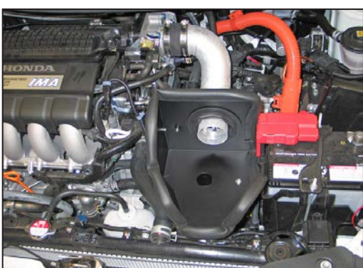
25. Install the heat shield/tube assembly into position and install the lower air duct onto the tube on the heat shield. Secure the heat shield to the factory airbox mounting locations with the hardware provided. Then secure the intake tube to the throttle body hose with the provided hose clamp.
