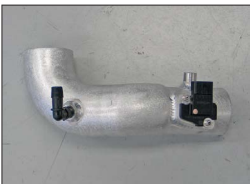
18. Install the provided 90° vent fitting into the K&N® intake tube as shown. NOTE: Plastic NPT fittings are easy to cross thread. Install the vent fitting “hand” tight, then turn it two complete turns with a wrench.
