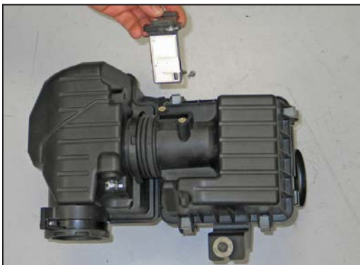
16. Remove the two screws securing the mass air sensor into the factory airbox, and then remove the mass air sensor.
