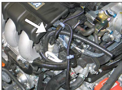
13. Route the provided bypass hose through the factory retaining clip as shown.
