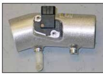
19. Install the provided 90°npt fitting into the K&N<sup>®</sup> intake tube as shown.
