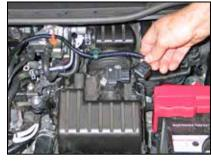
2. Disconnect the mass air sensor electrical connection and unhook the wiring harness from the factory air box.
