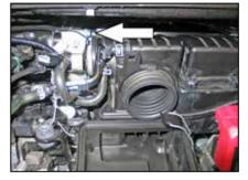
5. Loosen the hose clamp which secures the air box to the throttle body.
