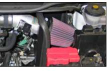
22. Install the K&N $^{\ensuremath{\$}}$  air filter and secure with the provided hose clamp.
