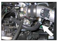
21. Install the provided crankcase vent hose onto the fitting installed onto the K&N<sup>®</sup> intake tube and then connect the open end to the valve cover vent port.
