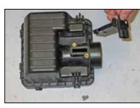
17. Remove the two screws securing the mass air sensor to the air box and then remove the mass air sensor as shown.
