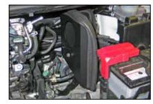
12. Install the heat shield assembly into position and secure to the previously installed bracket with the hardware provided.
