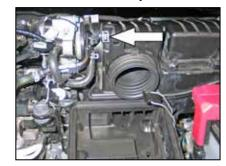
6. Release the spring clamp which secures the crank case vent hose to the air box and then disconnect the crankcase vent hose.
