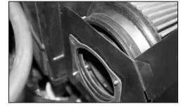
20. Place the gasket on the heat shield, as shown.
