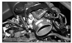
17. Attach the silicone hose to the throttle body with the hose clamps provided.
