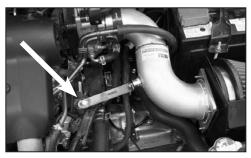
23. Install the "L" bracket and secure with the provided hardware.
