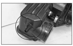
9. Remove the air temperature sensor from the factory airbox.
