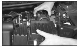
8. Remove the factory airbox by pulling away from the throttle body and lifting upwards.
