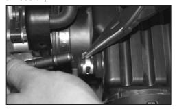
3. With pliers, depress the hose clamp and remove the crankcase vent (CCV) hose.
