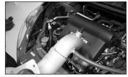
19. Install the other end of the silicone hose to the vent line on the K&N® intake tube.
