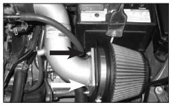
22. Secure the K&N<sup>®</sup> intake tube to the heat shield using the provided hardware.
