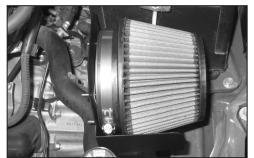
16. Place the filter assembly on the heat shield as shown. Tighten the lock nut on the vibration mount. NOTE: Heat shield should be perpendicular (90 degrees) to the battery. It may be necessary to loosen the battery and move it back to gain clearance for the heat shield
