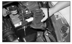
5. Separate the fresh air duct from the factory intake and completely remove.
