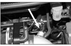
24. Clip the ATS harness into the air temperature sensor.
