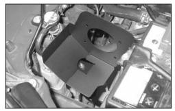
15. Place the heat shield onto the rubber mounted stud, then place the provided hardware. Pivot the heat shield around.
