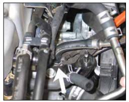
10. Ensure that the engine is not hot, then release the spring clamp that secures the coolant bypass hose to the intake manifold port. Disconnect the coolant bypass hose from the intake port. **NOTE: Ensure the engine is cool before disconnecting the coolant bypass hose. Capture any lost coolant.**
