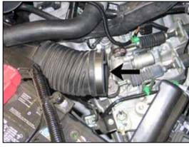
24. Install the provided hose clamp onto the stock fresh air supply hose as shown.
