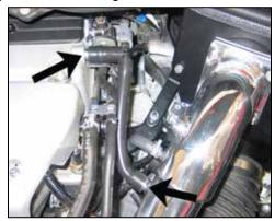
29. Install the crankcase vent hose assembly onto the valve cover port and intake tube port as shown and secure it with the provided hose clamp.
