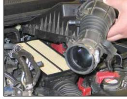
5. Release the six upper airbox clips, then remove the upper airbox and intake tube assembly as shown.
