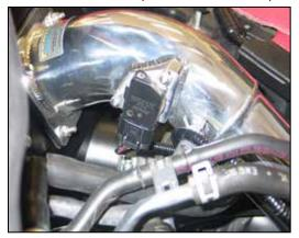
30. Re-connect the mass air sensor electrical connection.
