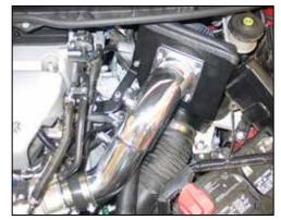
25. Install the intake assembly into the silicone hose at the throttle body and align the mounting bracket with the airbox mounting stud. Secure the intake assembly with the provided hose clamp and the factory nut that was removed in step #6. Secure the fresh air tube to the heat shield with the hose clamp.
