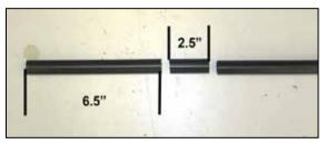
27. Using a knife, cut the provided crankcase vent hose in 2.5" and 6.5" pieces as shown.
