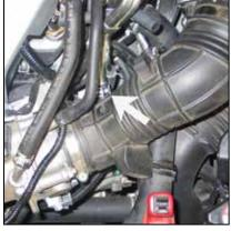
4. Release the crankcase breather hose spring clamp. Release the hose clamp that secures the intake tube to the throttle body.
