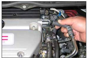
9. Release the spring clamp that secures the crankcase vent hose to the valve cover, then disconnect the crankcase vent hose from the valve cover.
