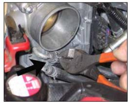
11. Release the spring clamp that secures the coolant bypass hose to the throttle body, then disconnect the coolant bypass hose from the throttle body. Remove the bypass/crank case vent hose assembly from the vehicle. NOTE: Ensure the engine is cool before disconnecting the coolant bypass hose. Capture any lost coolant.
