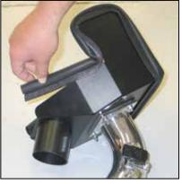
19. Install the provide edge trim onto the heat shield as shown. NOTE: Some trimming of the edge trim may be necessary.
