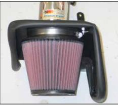
21. Install the  $K\&N^{\mathbb{R}}$  air filter onto the air filter adapter and secure with the provided hose clamp.
