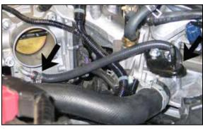
12. Install the provided bypass hose onto the throttle body and intake manifold ports. Secure with the provided hose clamps.
