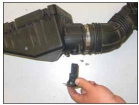
13. Remove the two screws that secure the mass air sensor to the upper airbox, then remove the mass air sensor as shown.
