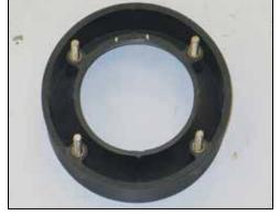
15. Install the four 6mm studs into the air filter adapter; threading them down until they bottom into the insert. tighten finger-tight.
