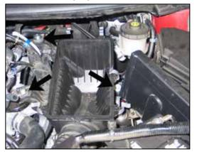
6. Remove the one nut and two bolts that secure the lower airbox to the vehicle. NOTE: This nut will be used again.
