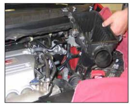
8. Remove the complete lower airbox assembly from the vehicle as shown.
