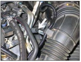
3. Release the spring clamp, then disconnect the EVAP canister hose from the intake tube as shown.
