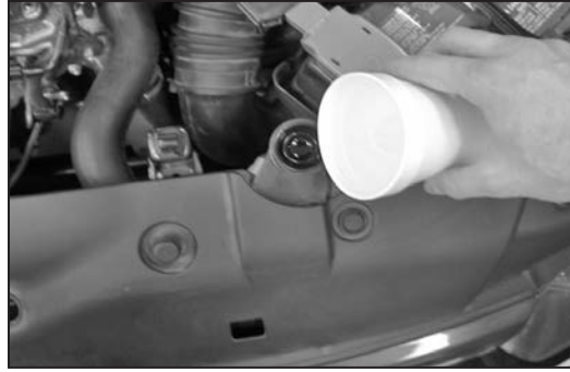
31. Loosen and remove the radiator cap to replace the coolant drained from step #11.
