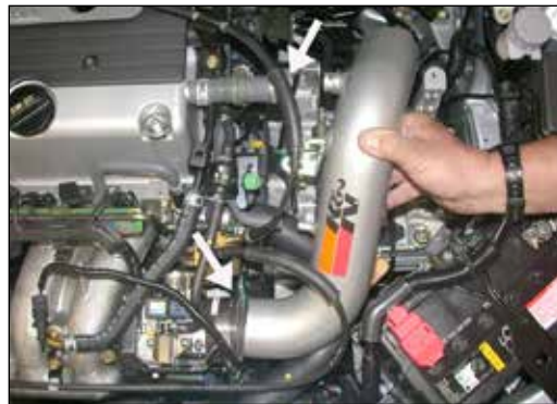
18. Install the second hose clamp onto the silicone hose, then, slide the K&N® intake tube into the silicone hose as shown. Line up the intake tube bracket with the original air cleaner mounting point.
