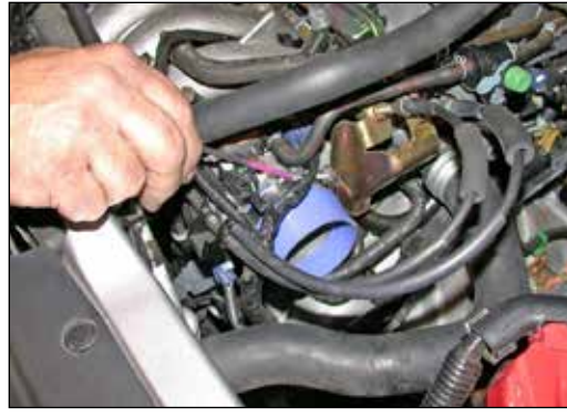
16. Install the silicone hose and hose clamp onto the throttle body as shown. NOTE: It may be necessary to fully open the hose clamp so it will slide over the throttle body.
