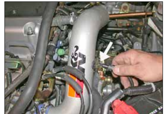
23. Push the air temperature sensor into the grommet on the K&N® intake tube as shown.
