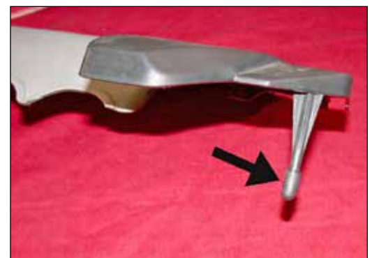
25. Install the rubber cap plug onto the stand off on the engine cover as shown.
