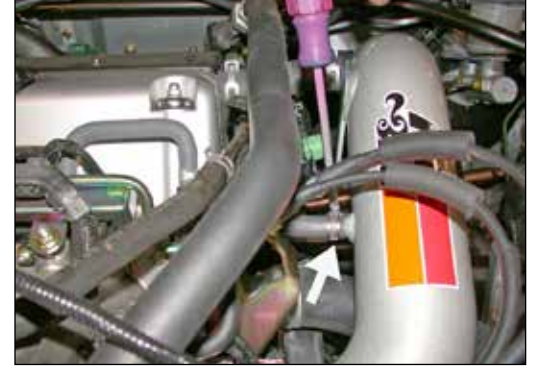
22. Reconnect the idle air bypass control thermal valve vent hose to the vent on the K&N® intake tube and secure with the provided hose clamp as shown.
