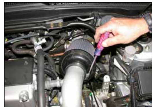
24. Install the K&N® air filter onto the K&N® intake tube and secure with the provided hose clamp as shown.
