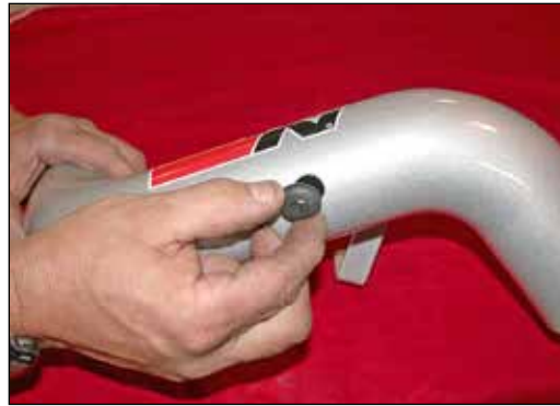
17. Install the provided grommet into the hole on the K&N® intake tube as shown.
