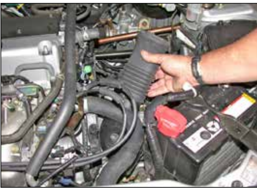
13. Remove the air inlet duct as shown. NOTE: K&N Engineering, Inc., recommends that customers do not discard factory air intake.
