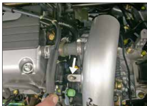
20. Using a 10mm socket secure the bracket to the air cleaner mounting point using the provided hardware.
