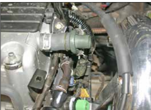
14. 2005-06 Model Year Vehicles ONLY: On '05-'06 models, remove the stock crank case vent hose as shown.
