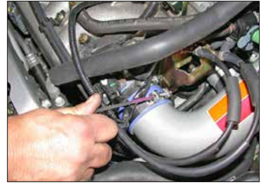
21. Using a flat blade screwdriver, tighten the hose clamp on the silicone hose as shown.
