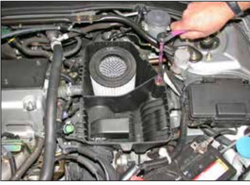
10. Loosen and remove the two bolts and one nut on the lower air cleaner assembly as shown.
