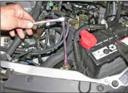
12. Using a 10mm socket, loosen the bolt that secures the air inlet duct as shown.
