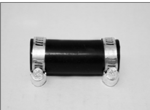
15. 2005-06 Model Year Vehicles ONLY: On '05-'06 models, place hose clamps on each side of the silicone hose (08692), as shown.
