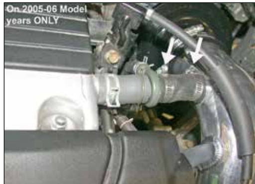
19. 2005-06 Model Year Vehicles ONLY: Using the supplied silicone hose and hose clamps, secure the silicone hose to the stock crank case vent line and to the vent tube on the intake tube as shown.
