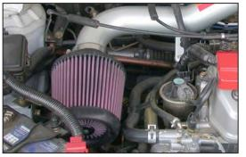
22. Install the K&N<sup>®</sup> air filter onto the K&N<sup>®</sup> intake tube and secure with the provided hose clamp. Adjust for best fit and clearance then tighten all hardware.
