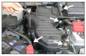
6. Loosen and remove the four bolts that secure the air intake resonator.
