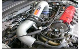
18. Install the K&N<sup>®</sup> intake tube onto the throttle body, then, line up the bracket with the rubber mounted stud as shown. Tighten hose clamps at this time.
