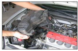
12. Unclip the throttle cable and cruise control cable (If equipped), then, remove the resonator by pulling upwards as shown.
