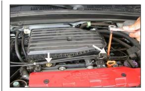
7. Loosen and remove the two bolts that secure the throttle body plenum.
