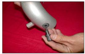
17. Install the provided rubber grommet into the hole on the K&N<sup>®</sup> intake tube, then install the air temperature sensor into the grommet as shown. NOTE: Before installing the grommet and air temperature sensor, Inspect the inside of the tube for any debris, then clean the inside out with water and a towel. Inspect the tube one more time before proceeding to the next step.
