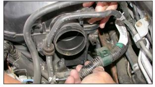
11. Using a flat blade screwdriver, unclip the wire harness from the resonator as shown.
