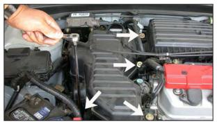
6. Loosen and remove the four bolts that secure the air intake resonator.
