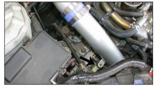
23. Slide the K&N<sup>®</sup> cold air tube onto the throttle body tube and line up the bracket with the rubber mounted stud as shown and secure with the provided hardware. Do not tighten completely.
