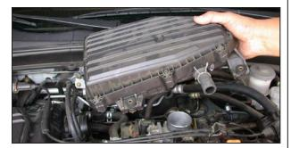
10. Pull firmly upwards to remove the throttle body plenum as shown.
