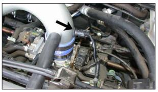
27. Reconnect the air temperature sensor electrical connection as shown.
