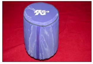
24. Install the K&N $^{\ensuremath{\mathbb{R}}}$  Drycharger $^{\ensuremath{\mathbb{R}}}$  onto the K&N $^{\ensuremath{\mathbb{R}}}$  air filter as shown.
