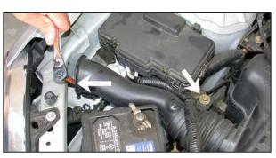
4. Loosen and remove the two bolts that secure the air inlet duct as shown.
