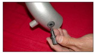
17. Install the provided rubber grommet into the hole on the K&N<sup>®</sup> intake tube, then install the air temperature sensor into the grommet as shown. NOTE: Before installing the grommet and air temperature sensor, inspect the inside of the tube for any debris, then clean the inside out with water and a towel. Inspect the tube one more time before proceeding to the next step. NOTE: Take care when handling the temp sensor as it is very fragile.
