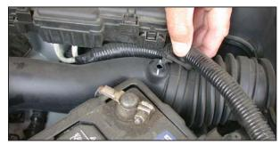
3. Unclip the battery cable from the air inlet duct as shown.
