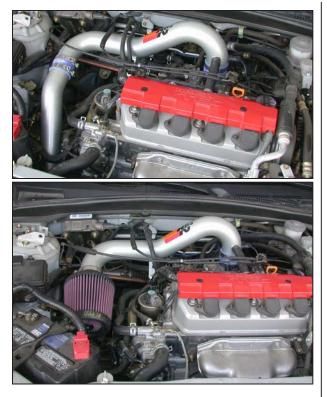
28. This K&N<sup>®</sup> high flow intake system has been designed to be used in two different configurations. In the case of inclement weather, the cold air tube can be removed and the air filter can be clamped onto the intake tube located in the engine compartment to avoid the possibility of ingesting water into the engine.
