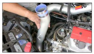
22. Install the tube as shown turning the tube in a clockwise rotation while inserting the tube in between the battery tray and the starter solenoid.
