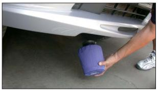
25. Raise the vehicle up and support it with jack stands, then, install the K&N<sup>®</sup> air filter from underneath the vehicle as shown.
