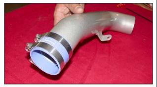
21. Install the silicone hose and hose clamps onto the K&N<sup>®</sup> cold air tube as shown.
