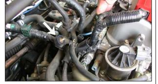
15. Install the rubber mounted stud onto the stock resonator mounting location as shown.
