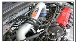
18. Install the K&N<sup>®</sup> intake tube onto the throttle body, then, line up the bracket with the rubber mounted stud as shown. Tighten hose clamps at this time.
