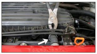
9. Using a pair of pliers, depress and pull back the hose clamp on the crank case vent at the cam cover.
