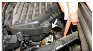
2. Disconnect the air temperature sensor electrical connection as shown.
