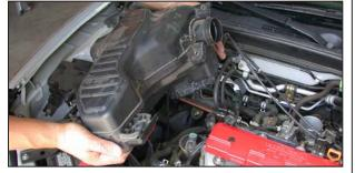
12. Unclip the throttle cable and cruise control cable (If equipped), then, remove the resonator by pulling upwards as shown.
