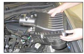
7. Remove the air filter assembly from the vehicle. NOTE: K&N Engineering, Inc., recommends that customers do not discard factory air intake.
