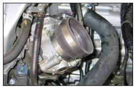
15. Install silicone hose number 084034 onto the throttle body and secure with the provided hose clamp.
