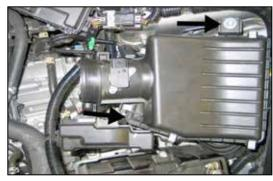
6. Loosen the two bolts securing the air box assembly to the inner fender and ECU bracket. 8. Remove the rear air filter mounting bracket shown from the strut tower.
