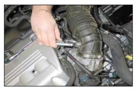
4. Release the spring clamp and disconnect the crank case vent tube from the intake tube.
