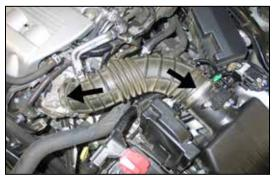
3. Loosen the hose clamps which secure the stock intake tube to the throttle body and air filter assembly.
