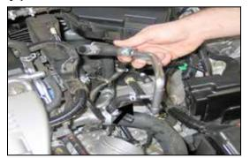
11. Release the spring clamp and then disconnect the steel by-pass hose assembly from the bypass hose attached to the thermostat housing. **NOTE: Be sure to capture any coolant that is released from the by-pass hose.**
