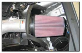
25. Install the K&N $^{\circ}$  filter and secure with provided hose clamp.
