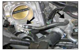
12. Connect the remaining bypass hose from the thermostat housing to the throttle body and secure with the factory hose clamp.
