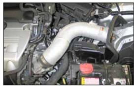
23. Install the K&N<sup>®</sup> intake tube through the heat shield, into the silicone hose at the throttle body and align with the tube mounting bracket previously installed. Align and then secure with the provided hose clamp and hardware.
