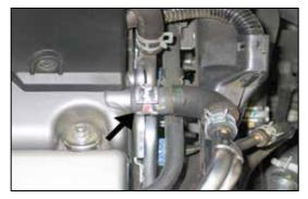
9. Release the spring clamp then unhook the crank case vent hose from the valve cover.
