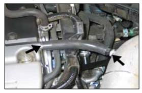
24. Install the provided crank case vent hose onto the valve cover vent port and fitting onto the K&N<sup>®</sup> intake tube.
