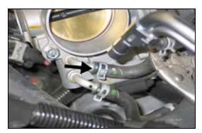
10. Release the spring clamp then remove the upper throttle body by-pass hose from the throttle body.
