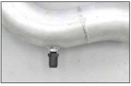
22. Install the provided NPT vent fitting into the intake tube as shown.
