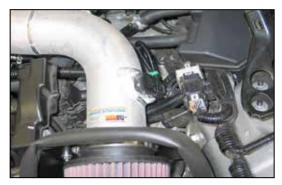
14. Secure bracket number 083121 to the thermostats housing as shown with the provided hardware.
