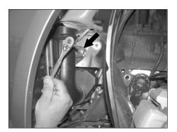
11. Loosen and remove the bolt that secures the resonator to the inner fender as shown.
