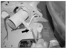
27. Secure the bracket on the cold air tube to the original resonator mounting hole using the provided hardware as shown.
