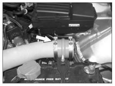
24. Install the silicone hump hose and hose clamps onto the  $K\&N^{\mbox{\tiny \ensuremath{\$}}}$  short ram tube as shown.
