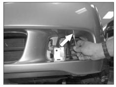
12. Loosen and remove the bolt secures the resonator to the inner fender as shown.
