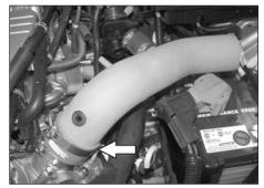
20. Slide the intake tube into the silicone hose on the throttle body as shown.
