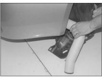
25. Install the cold air tube from underneath the vehicle as shown.
