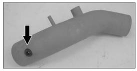
17. Install the provided grommet into the K&N<sup>®</sup> short ram tube as shown.
