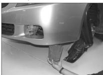
29. Install the filter from underneath the vehicle and secure it using the provided hose clamp.
