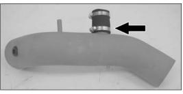
18. Install the silicone hose and hose clamps onto the vent on the  $K\&N^{\otimes}$  short ram tube as shown.
