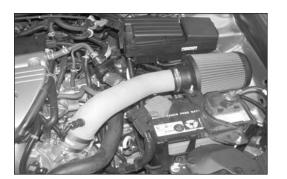
33. This K&N<sup>®</sup> high flow intake system has been designed to be used in two different configurations. In the case of inclement weather, the cold air tube can be removed and the air filter can be clamped onto the intake tube located in the engine compartment to avoid the possibility of ingesting water into the engine.
