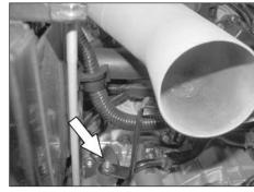
21. Line up the "Z" bracket with the rubber mounted stud and secure with the provided hex nut as shown, but do not tighten at this time.
