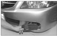
8. Remove the air inlet cover as shown.
