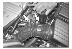
2. Disconnect the crankcase vent hose and the EVAP vent hose from the stock intake tube as
