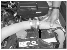
26. Slide the cold air tube into the silicone hump hose as shown.
