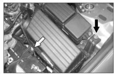
5. Loosen the two bolts on the stock air cleaner as shown.
