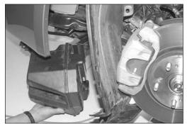
14. Remove the resonator as shown.
