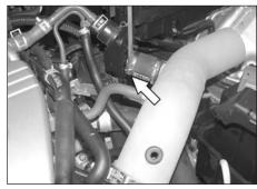
22. Reconnect the EVAP vent and the crankcase vent hose to the K&N<sup>®</sup> short ram tube as shown.
