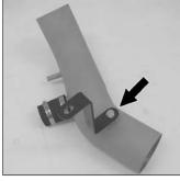
19. Using the provided hardware install the long end of the provided "Z" bracket onto the threaded boss on the K&N<sup>®</sup> short ram tube as shown.
