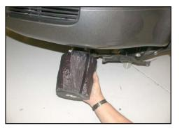
32. Install the K&N<sup>®</sup> air filter from underneath the vehicle and secure it with the provided hose clamp as shown.
