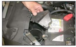
3. Use a flat blade screwdriver to remove the air inlet cover, which is secured by two plastic rivets. 5. Unclip the wire harness from the stock intake tube as shown.
