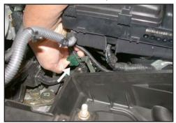
9. Depress the release tab and remove the wire harness from the bracket on the lower air cleaner assembly as shown.
