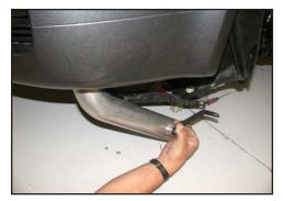
28. From underneath the vehicle slide the K&N<sup>®</sup> cold air intake tube through the hole in the inner fender as shown.
