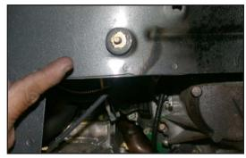
26. Install the provided rubber mounted stud into
