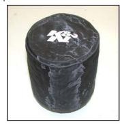
31. Install the K&N $^{\mbox{\tiny B}}$  Drycharger $^{\mbox{\tiny B}}$  onto the K&N $^{\mbox{\tiny B}}$  air filter as shown.
