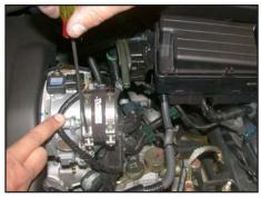
19. Install the silicone hose and hose clamps onto the throttle body and tighten as shown.
