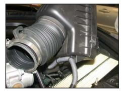
7. Loosen the four bolts on the air cleaner cover and pull upwards, then, unclip the wire harness and remove the cover as shown.
