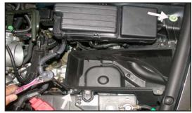
2. Pull firmly upwards to remove the battery cover, then, disconnect the negative battery cable.
