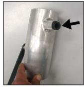
22. Install the silicone hose into the vent on the  $K\&N^{\otimes}$  short ram intake tube as shown.
