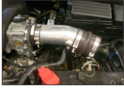
25. Slide the silicone hump hose onto the K&N<sup>®</sup> short ram intake tube as shown, but do not tighten at this time.
