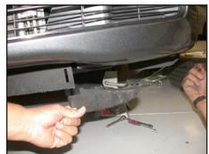
12. Remove the lower spoiler flap which is secured by two bolts as shown
