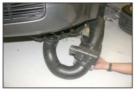
18. Remove the two bolts that secure the resonator to the inner fender, then, remove the resonator as shown.
