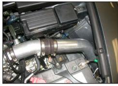
29. Slide the K&N<sup>®</sup> cold air intake tube into the silicone hump hose as shown, then tighten the hose clamps.
