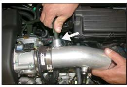
23. Slide the K&N<sup>®</sup> short ram intake tube into the silicone hose on the throttle body, then, slide the crankcase vent hard line into the vent on the intake tube as shown, but do not tighten at this time.
