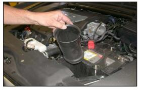
15. Remove the upper air inlet duct as shown.
