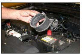
14. Remove rubber coupler from resonator tube
