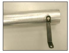
27. Install the provided bracket onto the threaded boss on the K&N<sup>®</sup> cold air intake tube and secure with the provided hardware as shown. **NOTE: Before installing the bracket, inspect the inside of the tube for any debris, then clean the inside out with water and a towel. Inspect the tube one more time before proceeding to the next step.**
