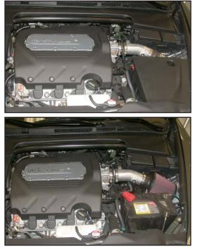
36. This K&N<sup>®</sup> high flow intake system has been designed to be used in two different configurations. In the case of inclement weather, the cold air tube can be removed and the air filter can be clamped onto the intake tube located in the engine compartment to avoid the possibility of ingesting water into the engine.
