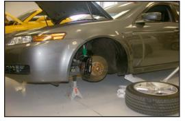
11. Raise the vehicle up and support it with jack stands, then, remove the front tire as shown.
