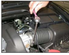
6. Loosen the hose clamp at the throttle body as shown.
