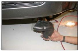
17. From underneath the vehicle remove the resonator inlet duct, which is secured by a bolt to the resonator.
