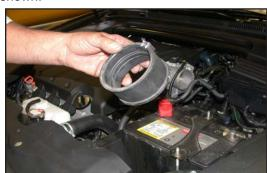
14. Remove rubber coupler from resonator tube assembly.
