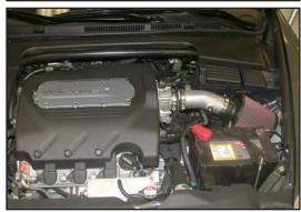
36. This K&N® high flow intake system has been designed to be used in two different configurations. In the case of inclement weather, the cold air tube can be removed and the air filter can be clamped onto the intake tube located in the engine compartment to avoid the possibility of ingesting water into the engine.
