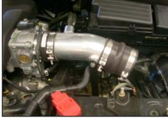
25. Slide the silicone hump hose onto the K&N® short ram intake tube as shown, but do not tighten at this time.
