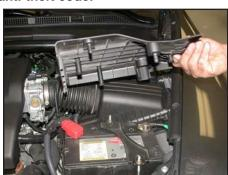
2. Pull firmly upwards to remove the battery cover, then, disconnect the negative battery cable.
