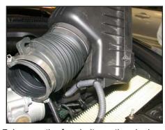
7. Loosen the four bolts on the air cleaner cover and pull upwards, then, unclip the wire harness and remove the cover as shown.
