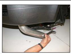
28. From underneath the vehicle slide the K&N® cold air intake tube through the hole in the inner fender as shown.
