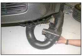
18. Remove the two bolts that secure the resonator to the inner fender, then, remove the resonator as shown.
