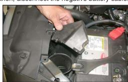
3. Use a flat blade screwdriver to remove the air inlet cover, which is secured by two plastic rivets.
