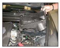
10. Slide the lower air cleaner assembly off of the air inlet duct and remove the lower air cleaner assembly as shown.
