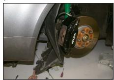
13. Remove one bolt and four plastic rivets, then, pull the inner wheel valance back and down as shown.
