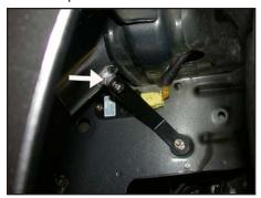
30. Line up the bracket with the rubber mounted stud in the inner fender, then, secure it using the provided hardware as shown.
