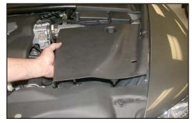
35. Reconnect the negative battery cable and double check to make sure everything is tightened and properly positioned before starting the vehicle. Reinstall the battery cover as shown.
