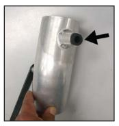
22. Install the silicone hose into the vent on the K&N® short ram intake tube as shown.
