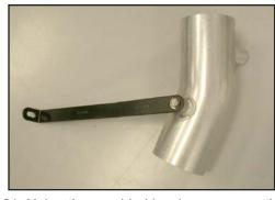
21. Using the provided hardware secure the provided bracket onto the  $K\&N^{\scriptsize @}$  short ram tube as shown.
