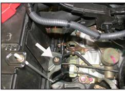
20. Install the provided rubber mounted stud into the original air cleaner mounting hole on the battery tray as shown.
