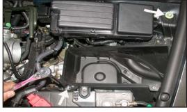
8. Loosen and remove the two bolts that secure the lower air cleaner assembly as shown.
