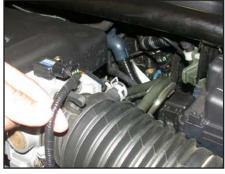
5. Unclip the wire harness from the stock intake tube as shown.
