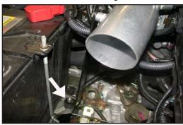
24. Secure the bracket to the rubber mounted stud and secure it with the provided hardware as shown but do not tighten at this time.
