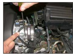
19. Install the silicone hose and hose clamps onto the throttle body and tighten as shown.
