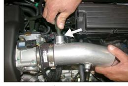
23. Slide the K&N® short ram intake tube into the silicone hose on the throttle body, then, slide the crankcase vent hard line into the vent on the intake tube as shown, but do not tighten at this time.
