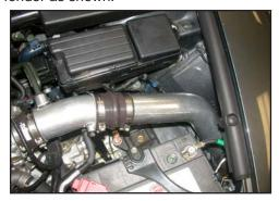
29. Slide the K&N® cold air intake tube into the silicone hump hose as shown, then tighten the hose clamps.
