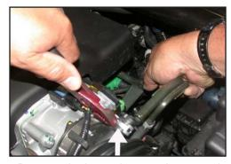
4. Depress the hose clamp and remove the crankcase vent hard line from the stock intake tube as shown.
