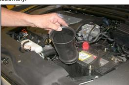
15. Remove the upper air inlet duct as shown.
