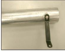
27. Install the provided bracket onto the threaded boss on the K&N® cold air intake tube and secure with the provided hardware as shown.
