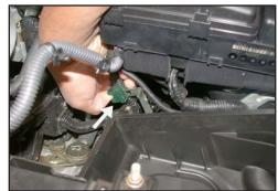
9. Depress the release tab and remove the wire harness from the bracket on the lower air cleaner assembly as shown.
