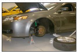
11. Raise the vehicle up and support it with jack stands, then, remove the front tire as shown.
