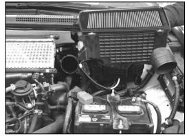
2. Loosen the four quarter turn fasteners that attach the engine cover and lift off the engine cover.
