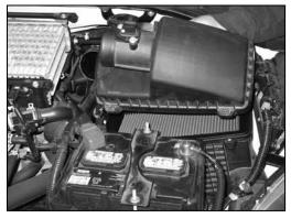
6. Loosen the four bolts that secure the upper airbox housing to the lower airbox housing and then remove the upper airbox housing.
