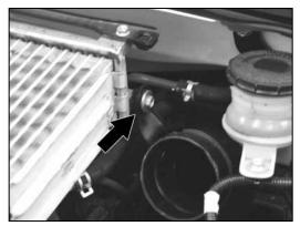
9. Remove the turbo inlet tube mounting bolt shown.
