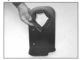
11. Install supplied short edge trim into the hole of the heat shield as shown. NOTE: Some trimming of the edge trim may be necessary.
