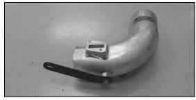
17. Install the supplied tube mounting bracket (070098) onto the K&N® intake tube using the provided hardware.
