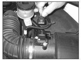
3. Disconnect the mass air sensor and unhook the wiring harness from the airbox and intake tube.
