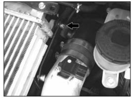
20. Install the K&N<sup>®</sup> intake tube into the silicone hose at the turbo inlet tube and align so the mounting bracket lines up with the turbo inlet mounting location. Secure the intake tube with the hose clamp and hardware provided.
