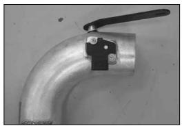
19. Install the mass air sensor into the K&N<sup>®</sup> intake tube and secure with the provided hardware.
