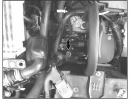
15. Secure the heat shield mounting bracket to the lower airbox mounting tab using the bolt removed in step #7. NOTE: Be sure to place the provided spacer between the bracket and mounting tab.
