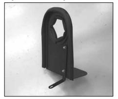
13. Install the "L" bracket (070097) onto the heat shield with the provided hardware.
