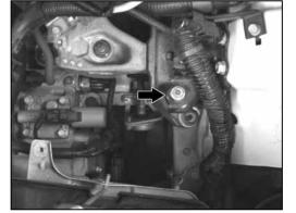
10. Remove the transmission mount bolt shown.
