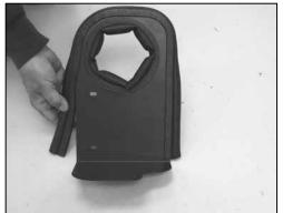
12. Install the long edge trim around the outside of the heat shield as shown. NOTE: Some trimming of the edge trim may be necessary.
