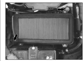
7. Remove the two lower airbox mounting bolts.
