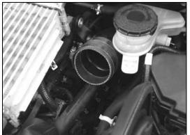
16. Install the provided silicone hose (08711) onto the turbo inlet tube and secure with the provided hose clamp.
