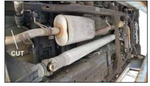
2. Unless a vehicle lift is available cutting the stock exhaust will be mandatory to remove. Cut rear tailpipe 2" from rear hanger just above the axle where shown.
