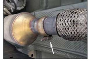
4. Once rear tail pipe has been removed loosen front conical clamp connecting tail pipe to head pipe.
