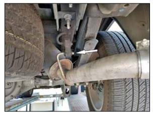
3. Remove rear tail pipe section by sliding tail pipe off rear hanger (leave rubber hanger on vehicle).
