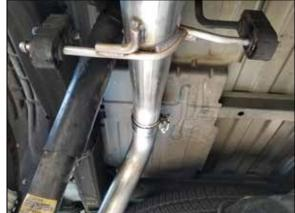
12. Slide band clamp on to the front of the tail pipe section. Then slide tail pipe section into muffler section.
