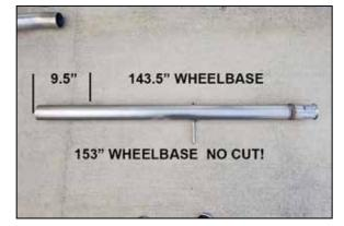
8. For vehicles with 143.5" wheelbase 9.5" must be cut off the end opposite to the conical end connecting to the head pipe (As shown). For vehicles with 153" wheelbase it does not need to be cut.
