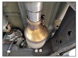
11. Slide mid pipe and muffler assembly into position on the vehicle by first using the hangers on the muffler end. Once inserted, then slide assembly rearward allowing the mid pipe to move into position to seat against head pipe with the factory conical clamp.
