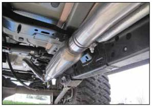
12. Install the K&N $^{\circ}$  muffler onto the K&N $^{\circ}$  mid pipe and into the factory hanger.
