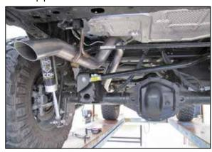
16. Check alignment and reposition as necessary. Once final position is satisfactory, tighten all band clamps from front to rear of vehicle.
