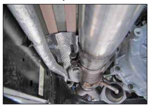
11. Install the  $K\&N^{\otimes}$  mid pipe to the factory catalyst pipe and secure with the factory clamp.
