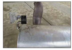
13. Remove the driver side muffler hanger from the stock muffler.
