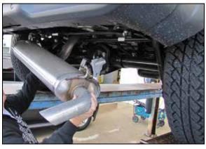
5. Using a twisting motion so the muffler pipe slides off the exhaust pipe, remove the muffler assembly from the vehicle.
