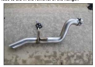
14. Install the driver side muffler hanger onto the K&N® tail pipe hanger.
