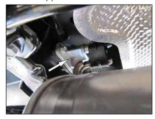
3. Loosen and remove the two bolts that secure the driver side muffler hanger to the chassis. **NOTE: one bolt is not in view in this picture.**
