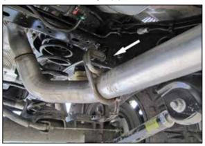
8. Disconnect the exhaust pipe hanger and then remove the exhaust pipe from the vehicle.
