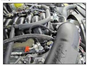
24. Connect the crank case vent hose and the fuel pressure hose to the fittings installed into the K&N<sup>®</sup> intake tube.
