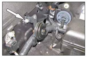
12. Remove the bolt which secures the horn to the inner fender.
