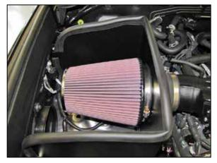
25. Install the K&N<sup>®</sup> air filter and secure with the provided hose clamp. **NOTE: Drycharger<sup>®</sup> air filter wrap; part #**
