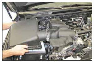
6. Release the four retaining clips securing the upper air box and then remove the upper air box and intake tube assembly from the vehicle.
