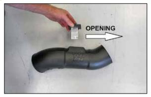
19. Install the mass air sensor assembly into the K&N $^{\circ}$  intake tube and secure with the provided hardware.
