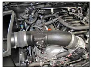
23. Install the K&N<sup>®</sup> intake tube into the hump hose at the heat shield and then into the step hose at the throttle body and secure with the provided hose clamp.
