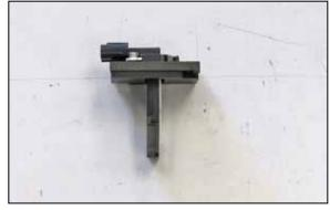
18. Install the mass air sensor assembly into the  $K\&N^{\mbox{\tiny @}}$  mass air sensor adapter as shown using the provided hardware.
