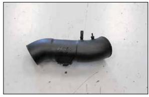
20. Install the provided NPT vent fittings into the  $K\&N^{\circledast}$  intake tube as shown.
