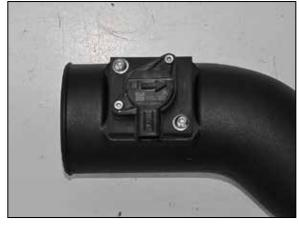
18. Install the mass air sensor assembly into the K&N<sup>®</sup> intake tube and secure with the provided hardware.
