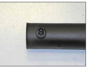
19. Install the provided NPT vent fitting into the  $K\&N^{\circledast}$  intake tube as shown.
