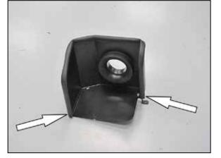
11. Install the provided edge trim onto the K&N<sup>®</sup> heat shield as shown.
