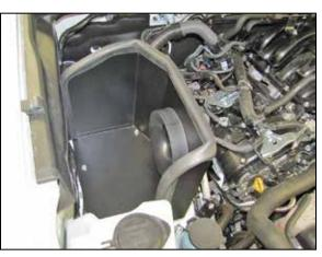
12. Install the heat shield onto the rubber mounted studs installed in the earlier step and secure with the provided hardware.
