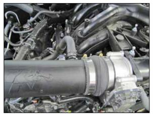
21. Connect the crank case vent fitting onto the vent fitting installed into the K&N<sup>®</sup> intake tube.
