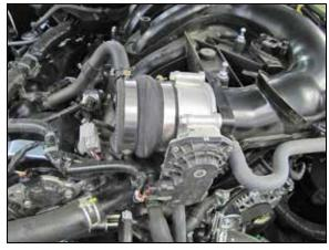
13. Install the provided coupler (01871) onto the throttle body and secure with the provided hose clamp.
