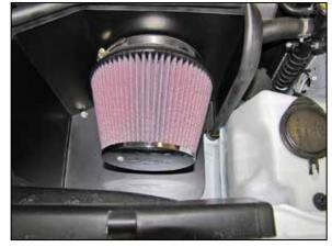
23. Install the K&N<sup>®</sup> air filter onto the filter adapter and secure with the provided hose clamp.
