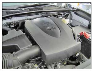
2. Lift up the engine cover to dislodge it from the mounting studs and then remove it from the vehicle. 3. Release the spring clamp and disconnect the crank case vent hose from the factory intake tube.
