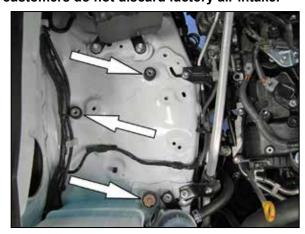
8. Install the three provided rubber mounted studs onto the inner fender in the positions shown.
