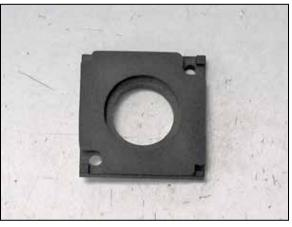
15. Install the provided gasket onto the  $K\&N^{\mbox{\scriptsize \$}}$  mass air sensor adapter.
