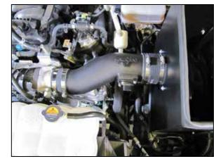
19. Install the provided coupler (08761) onto the intake tube (Do not tighten). Install the intake tube into the coupler at the throttle body and align with the filter adapter. Secure the coupler hose and intake tube with the provided hose clamps.
