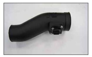
18. Install the mass air sensor assembly into the K&N® intake tube and secure with the provided hardware.
