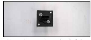
16. Remove the mass air sensor from the factory housing and install it into the K&N® mass air sensor adapter and secure with the provided hardware.
