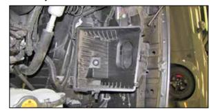
6. Remove the bolt that secures the lower air filter housing to the inner fender and then remove the lower air filter housing from the vehicle.
