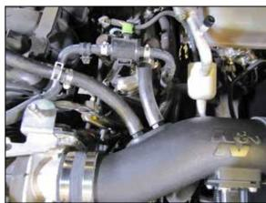
21. Install the vent fittings into the factory vent hoses and then onto the fittings installed into the K&N® intake tube.
