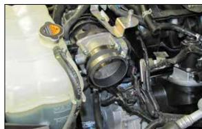
17. Install the provided coupler hose (08698) onto the throttle body and secure with the provided hose clamp.
