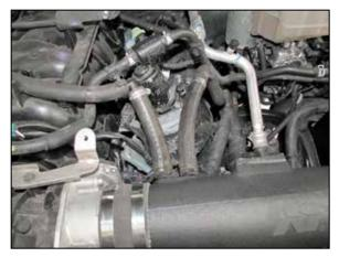
23. Install the vent hose assemblies into the factory vent hoses as shown; secure the factory vent hoses to the unions with the factory spring clamps. Connect the open ends of the hoses to the fittings installed into the K&N® intake tube.
