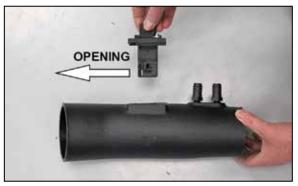
19. Install the mass air sensor assembly into the K&N<sup>®</sup> intake tube so that the opening in the sensor is towards the inlet end of the tube and then secure it with the provided hardware.
