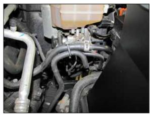
25. On 4 wheel drive vehicles, using one of the provided tie wraps secure the front differential breather to the EVAP lines.
