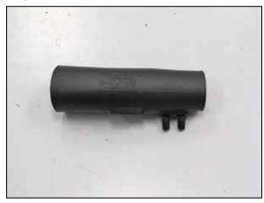
15. Install the two provided NPT vent fittings into the K&N<sup>®</sup> intake tube as shown. **NOTE: Plastic NPT fittings are easy to cross**
