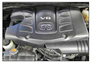
2. Remove the two bolts that secure the decorative engine cover and then remove the cover from the engine.
