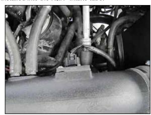
24. Reconnect the mass air sensor electrical connection.
