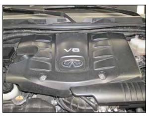
27. Install the decorative engine cover and secure with the factory hardware.
