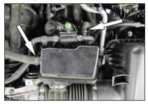
4. Release the spring clamps that secure the crank case breather hoses to the plenum chamber and then disconnect the crank case vent hoses. Unhook the EVAP canister from the plenum chamber.
