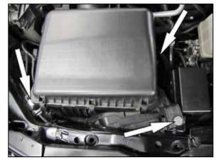
6. Remove the three bolts that secure the air filter housing to the inner fender and then remove the complete intake system from the vehicle. **NOTE: On 4 wheel drive applications it is necessary to unhook the front differential vent hose from the air filter housing.**
