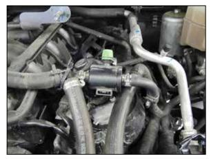
26. Using one of the provided tie wraps, secure the EVAP vent line to the crank case vent lines.
