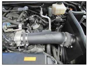
20. Install the K&N<sup>®</sup> intake tube into the hump coupler and then into the coupler at the throttle body, adjust the tube for best fit and then secure with the provided hose clamps.
