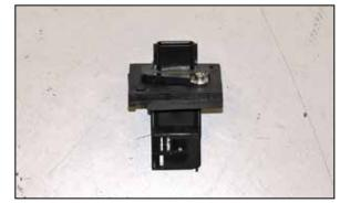
18. Install the mass air sensor into the K&N<sup>®</sup> adapter and secure with the provided hardware.
