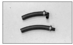
22. Install the provided union fittings into the vent hoses as shown and secure with the provided clamps. The 90° fitting will be installed into the 5" long hose.
