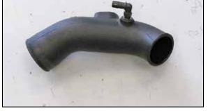
16. Install the provided 90° NPT vent fitting into the K&N<sup>®</sup> intake tube as shown. NOTE: Plastic NPT fittings are easy to cross thread. Install the vent fitting "hand" tight, then turn it two complete turns with a wrench. 21. Install the provided crank case vent hose onto the fitting in the intake tube and then onto the fitting on the valve cover.
