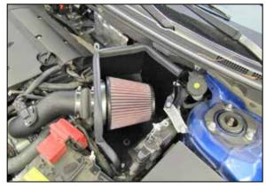
23. Install the K&N<sup>®</sup> air filter and secure with the provided hose clamp.
