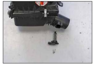
17. Remove the mass air sensor from the factory air filter housing.
