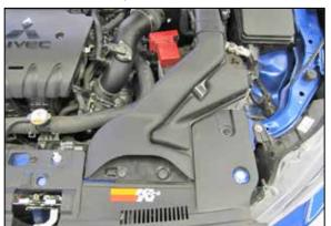
24. Reinstall the fresh air intake scoop and secure with the factory fasteners.
