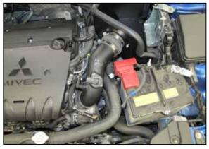
20. Install the K&N<sup>®</sup> intake tube into the coupler on the filter adapter and then into the coupler on the throttle body. Adjust the tube for best fit and then secure with the provided hose clamps.
