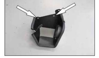
11. Install the two provided grommets into the heat shield as shown.
