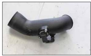
19. Using the four provided washers, install the mass air sensor into the K&N $^{\circ}$  intake tube and secure with the provided hardware.
