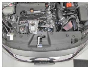
22. Reinstall the core support cover and secure with the factory retaining clips.
