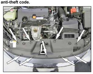
2. Remove the nine clips that secure the core support cover and then remove the cover from the vehicle.
