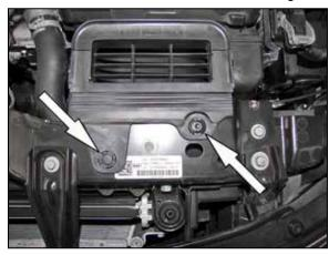
4. Remove the two plastic clips that secure the intake air diverter and then lift off the air diverter.
