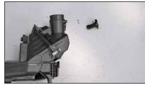
16. Remove the mass air sensor from the factory air filter housing.
