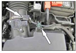
3. Disconnect the mass air sensor connection and unhook the harness from the air filter housing.
