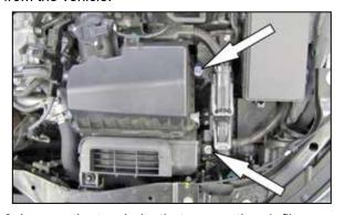
6. Loosen the two bolts that secure the air filter housing, apply some spray lubricant to the mounting grommet and then remove the air filter housing from the vehicle.
