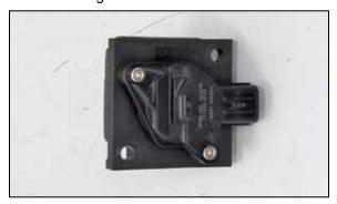
17. Install the mass air sensor into the K&N® mass air adapter and secure with the provided hardware.
