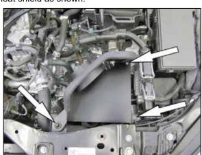
11. Install the heat shield assembly into the vehicle and secure with the provided hardware and factory grommet.
