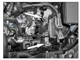
7. Install the two provided rubber mounted studs onto the air filter housing mounting locations as shown.
