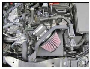
13. Install the coupling hose (087121) onto the filter adapter and secure with the provided hose clamp.
