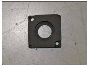
12. Install the provided gasket onto the mass air sensor adapter.
