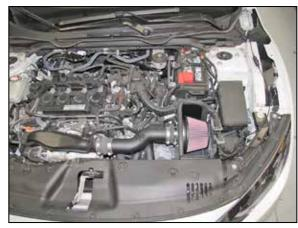
18. Reconnect the vehicle's negative battery cable. Double check to make sure everything is tight and properly positioned before starting the vehicle.
