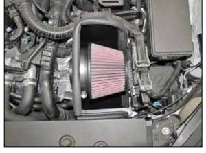
9. Install the filter assembly into the heat shield and secure with the provided hardware.
