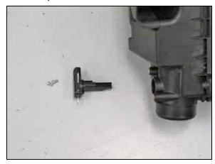
13. Remove the mass air sensor from the factory air filter housing.
