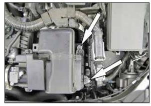
3. Loosen the two bolts securing the air filter housing to the mount bracket and inner fender.
