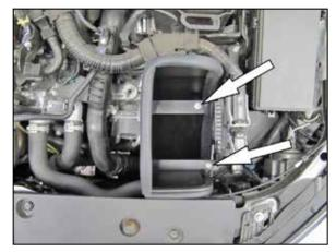
7. Install the heat shield onto the rubber mounted stud and air filter housing mounting bracket and secure with the provided hardware.
