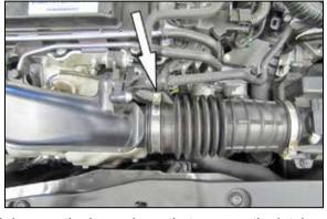
4. Loosen the hose clamp that secures the intake hose to the turbo inlet pipe and then remove the air filter housing and hose assembly.
