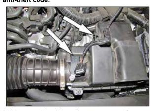
2. Disconnect the Mass air sensor connection and unhook the wiring harness from the air filter housing.
