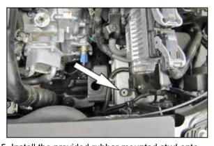
5. Install the provided rubber mounted stud onto the inner fender air filter housing mounting location.
