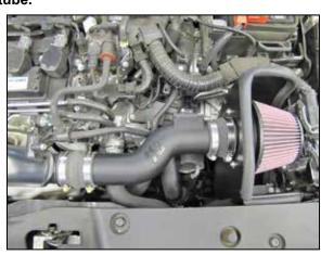
16. Install the K&N® intake tube assembly into the coupling hoses, adjust the tube for best fit and then secure with the provided hose clamps.
