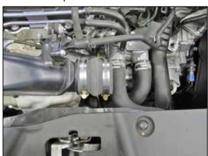
10. Install the coupling hose (084018) onto the turbo inlet pipe and secure with the provided hose clamp.
