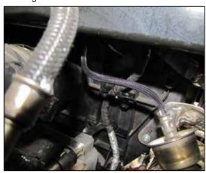
13. Disconnect the wiring harness's that attach to the rear of the air filter assembly.
