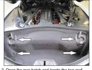
2. Open the rear hatch and locate the two roof stowage mounts. Remove the bolts that secure the stowage mounts and set the mounts aside. Remove the two wing nuts at the bottom of the compartment that secure the carpet.
