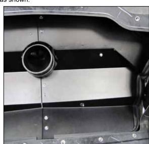
28. Set the intake tube into position but do not secure. Install the passenger side heat shield and align with the mounting bracket. Install all of the mounting hardware loosely before tightening. Reconnect the temperature sensor electrical connection.
