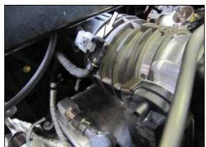
8. Disconnect the mass air sensor electrical connection.
