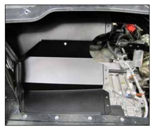
25. Install the drivers side heat shield assembly and align with the mounting bracket. Secure the heat shield with the provided hardware. Reconnect the "F" antenna electrical connection.
