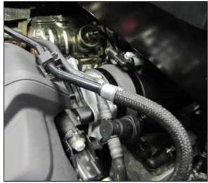
31. Reconnect the mass air sensor electrical connection.
