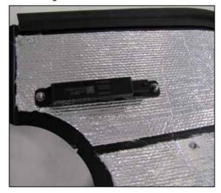
24. Install the "F" antenna to the engine side of the driver's side heat shield assembly using the provided hardware with the button head of the bolt on the filter side of the heat shield.
