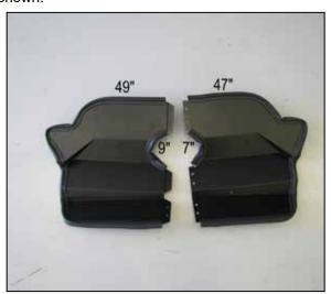
20. Install the provided edge trim onto the two heat shield halves as shown.
