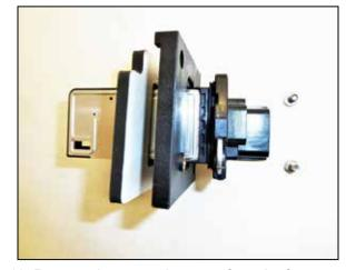
13. Remove the mass air sensor from the factory air filter housing. Assemble the mass air sensor, adapter and gasket as shown.
