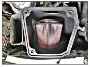
8. Set the K&N air filter into the filter housing.
