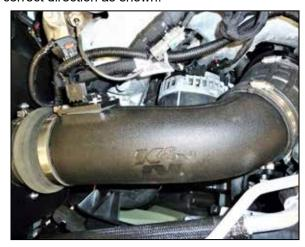
15. Install the K&N intake tube assembly into the coupler at the filter adapter and then into the factory coupler, adjust the tube for best fit and secure with the hose clamps.
