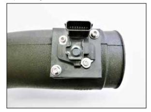
14. Install the mass air sensor assembly into the K&N intake tube and secure with the provided hardware. Be sure to install the sensor in the correct direction as shown.
