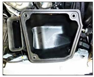
7. Set the K&N air filter housing into the vehicle so the studs protrude into the factory mounting grommets. Secure the K&N Air filter housing with the facory from step #4.
