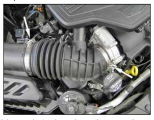
4. Loosen the two hose clamps that secure the factory intake hose. Remove the factory intake hose from the vehicle.
