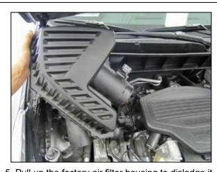
from the mounting grommets and then remove the housing from the vehicle.
