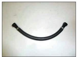
24. Install the provided quick connect fittings into the provided crank case vent hose and secure with
