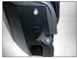
12. Install the provided wiring connector mounting bracket onto the heat shield using the provided hardware. Install the factory mounting grommet into the heat shield as shown.
