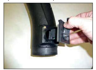
22. Install the mass air sensor into the  $K\&N^{\otimes}$  intake tube and secure with the provided hardware.
