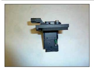
21. Install the provided gasket onto the K&N<sup>®</sup> mass air adapter. Remove the mass air sensor from the factory housing and install it into the mass air adapter and secure with the provided hardware.
