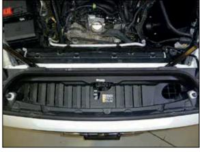
16. Reinstall the radiator valence and secure with the ten factory clips.
