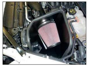
27. Install the K&N<sup>®</sup> air filter onto the adapter and secure with the provided hose clamp.
