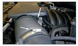
4. Loosen the hose clamps that secures the intake plenum to the air filter housing and to the throttle body. Disconnect the plenum connections at the air filter housing and then rotate the plenum counter clockwise to disengage the keyed mount and separate it from the throttle body. NOTE: The wiring harness anchored to the intake plenum will need to be detached before removing the plenum from the vehicle.
