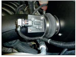
26. Connect the mass air sensor electrical connection.
