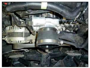
19. Install the provided reducer coupler onto the throttle body and secure with the provided hose clamp.
