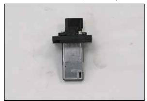
11. Remove the mass air sensor from the factory air filter housing. Install the sensor and provided gasket onto the K&N<sup>®</sup> filter adapter as shown.
