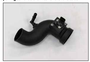
13. Install the provided quick disconnect fitting into the K&N<sup>®</sup> intake tube as shown.
