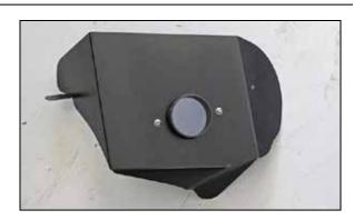
5. Install the provided filter adapter into the heat shield and secure with the provided hardware.
