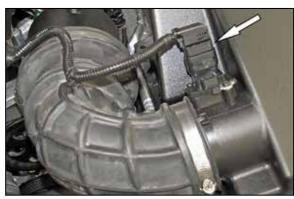
2. Disconnect the mass air sensor electrical connection and unhook the wiring harness from the intake tube.
