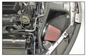
10. Install the heat shield/filter assembly into the vehicle so the mounting studs insert into the mounting grommets.
