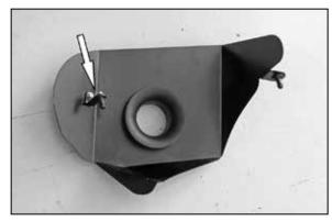
7. Install the remaining mounting stud onto the long leg of the provided "L" bracket (064340) and secure with the provided hardware, then install the assembly onto the heat shield as shown using the provided hardware.
