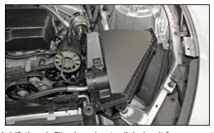
4. Lift the air filter housing to dislodge it from mount grommets and then remove the housing from the vehicle.
