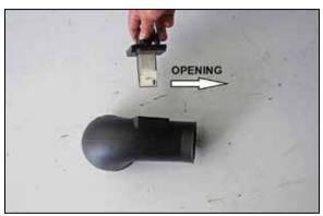
16. Install the mass air sensor assembly into the K&N® intake tube and secure with the provided hardware.
