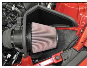
18. Install the K&N® air filter and secure with the provided hose clamp.
