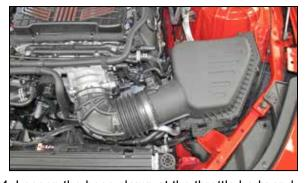
4. Loosen the hose clamp at the throttle body and then remove the complete stock intake system.
