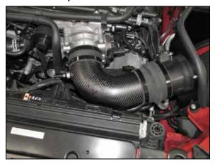
15. Install the K&N® intake tube assembly into the hump coupler and then into the coupler at the throttle body, adjust the tube for best fit and then secure with the provided hose clamps.
