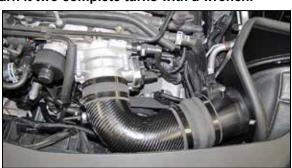
17. Install the intake tube assembly into the hump coupler and then into the coupler at the throttle body, adjust the tube for best fit and then secure with the provided hose clamps.
