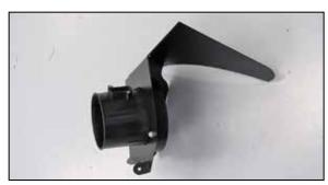
7. Install the K&N® mass air housing into the heat shield and secure with the provided hardware.
