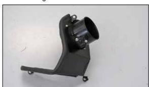
12. Install the mass air sensor into the K&N® air filter housing and secure with the provided hardware
