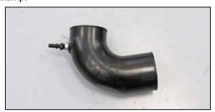
16. Install the provided NPT quick disconnect fitting into the  $K\&N^{\odot}$  intake tube.
