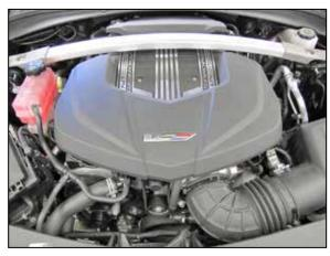
2. Lift the decorative engine cover and remove it from the engine.
