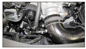
18. Connect the crank case vent fitting to the quick disconnect fitting installed into the K&N® intake tube.
