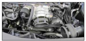
15. Install the provided coupler hose (08618) onto the throttle body and secure with the provided hose clamp.
