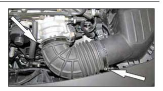
5. Loosen the hose clamps that secure the factory intake hose to the throttle body and air filter housing.
