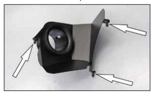
8. Install the provided heat shield mounting posts onto the heat shield and secure with the provided hardware.
