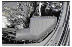
6. Lift the air filter housing assembly and remove it from the vehicle.
