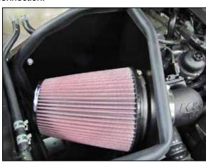
26. Install the K&N $^{\!0}$  air filter and secure with the provided hose clamp.
