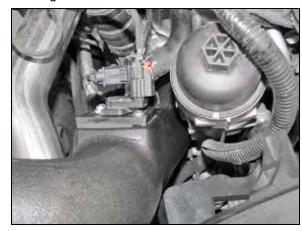
25. Reconnect the mass air sensor electrical connection.
