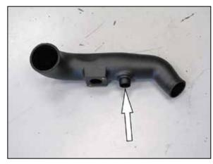
17. Install the provided grommet and quick disconnect fitting into the K&N® intake tube.
