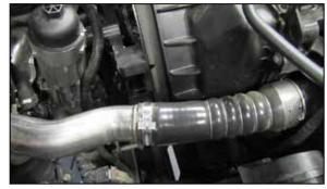
9. Loosen the charge tube flex hose and rotate it inwards  $90^{\circ}$  as shown and then retighten the clamp.
