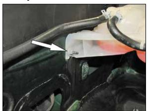
15. Remove the nut shown that secures the coolant reservoir.
