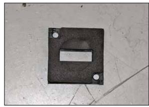
19. Install the gasket on to the K&N $^{\!0}$  mass air sensor adapter.
