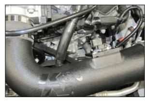
28. Install the provided crank case vent hose onto the factory vent hose and K&N® fitting.
