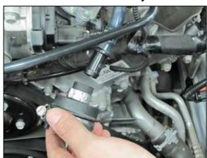
11. Remove the factory crank case vent coupler from the crank case vent tube.
