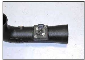
22. Install the mass air assembly into the  $K\&N^{\circledast}$  intake tube as shown.
