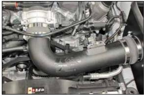
26. <u>Install the intake tube assembly</u> into the coupler at the filter adapter and then into the coupler on the throttle body, adjust the tube for best fit and then secure with the provided hose clamps.
