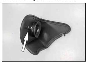
15. Install remaining mounting post onto the long leg of the provided bracket (064346) and then install the assembly onto the heat shield using the provided hardware.
