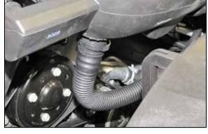
4. Release the sound tube quick disconnect fitting and disconnect the sound tube from the factory intake tube.
