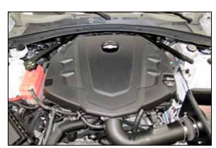
31. Reinstall the decorative engine cover and secure with the factory bolt and oil cap.
