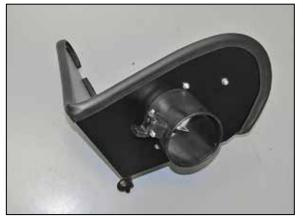
19. Install the mass air sensor into the K&N<sup>®</sup> mass air housing and secure with the provided hardware.
