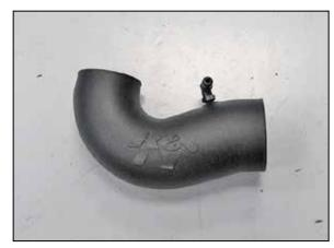
24. Install the provided 90° fitting into the K&N intake tube as shown.
