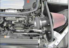
23. Install the K&N<sup>®</sup> air filter onto the filter adapter and secure with the provided hose clamp.
