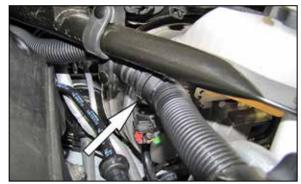
9. Disconnect the sound tube quick disconnect fitting and remove the complete sound tube system.
