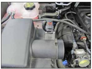
6. Disconnect the mass air sensor electrical connection.
