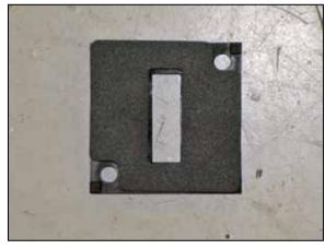
15. Install the provided gasket onto the K&N® mass air sensor adapter.
