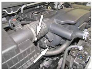
2. Loosen the two hose clamps that secure the intake plenum to the throttle body and air filter housing.
