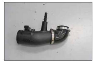
20. Install the provided angled coupling hose (084087) onto the intake tube as shown.
