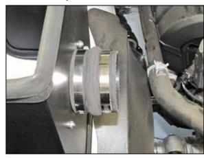
19. Install the provided coupling hose (08699) onto the filter adapter and secure with the provided hose clamp.
