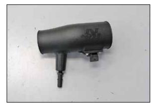
18. Install the Provided NPT quick disconnect fitting into the K&N® intake tube as shown.
