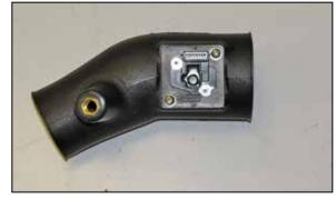
17. Install the mass air sensor into the K&N® adapter and then install the assembly into the K&N® intake tube and secure with the provided hardware.
