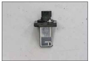
19. Install the mass air sensor into the K&N® mass air adapter.
