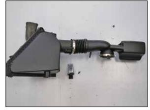
18. Remove the sensor from the factory intake system.
