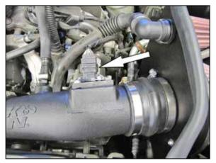
24. Connect the mass air sensor electrical connection.
