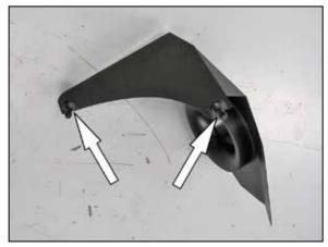
9. Install the two provided mounting studs onto the heat shield using the provided hardware.
