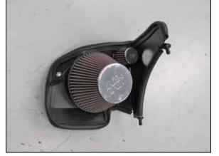
14. Install the K&N<sup>®</sup> air filter onto the filter adapter and secure with the provided hose clamp. NOTE: Drycharger<sup>®</sup> air filter wrap; part # 22-8049DK is available to purchase separately.
