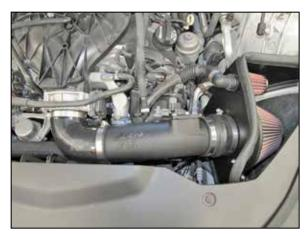
22. Install the intake tube onto the filter adapter first and then onto the throttle body. Adjust the tube and hoses for best fit and then secure with the provided hose clamps.
