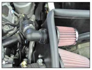
25. Connect the air injection hose to the quick disconnect fitting.
