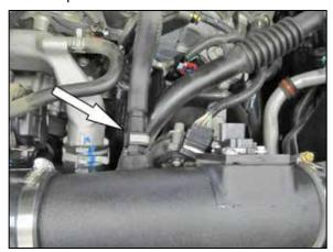
23. Connect the crank case vent hose to the quick disconnect fitting installed into the K&N<sup>®</sup> intake tube.
