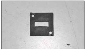
17. Install the provided gasket onto the mass air sensor adapter.
