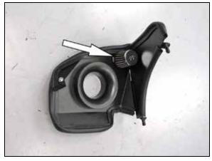
13. Install the quick connect adapter and crank case breather filter onto the heat shield as shown.
