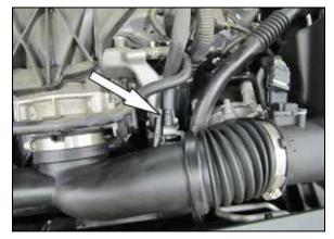
4. Release the clip securing the crank case vent line to the factory intake hose and then disconnect the crank case vent hose.
