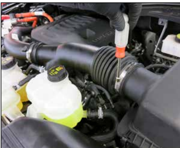
2. Loosen the three hose clamps that secure the intake tube.
