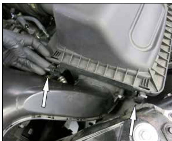
4. Release the two clips that secure the upper air filter housing to the lower air filter housing.
