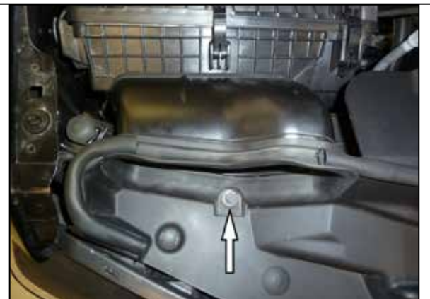
5. Remove the push pin securing the fresh air intake duct and then remove the duct from the vehicle.
