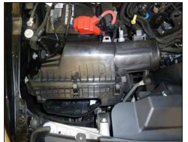
6. Pull up the air filter housing and remove it from the vehicle.
