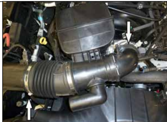
3. Loosen the two hose clamps securing the factory intake tube and then remove the intake tube from the vehicle.
