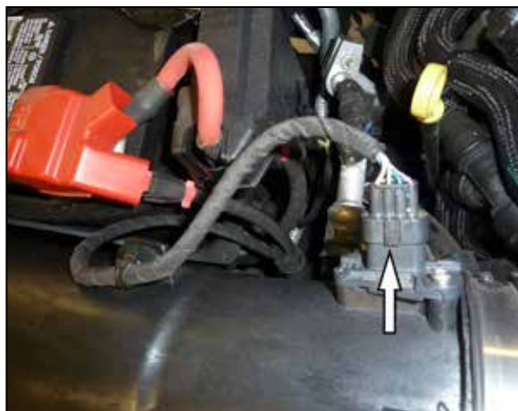
4. Disconnect the MASS air sensor electrical connection.
