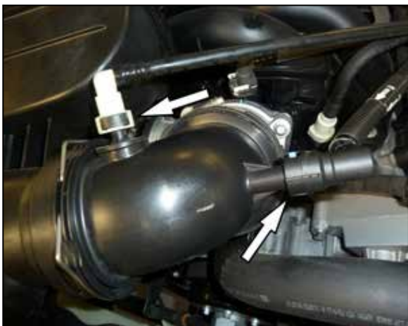
2. Disconnect the two CCV hoses from the factory intake tube.
