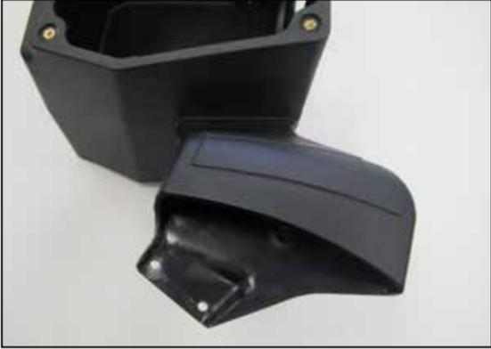
8. Install the K&N Fresh air intake duct to the K&N air filter housing and secure with the provided hardware.
