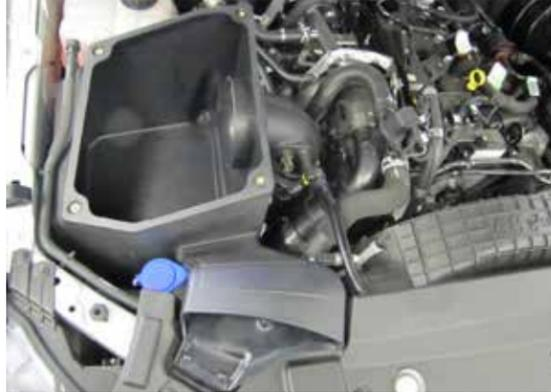
13. Install the provided Coupler hose (08711) onto the K&N intake tube and then install the complete assembly into the vehicle. Secure the housing and fresh air duct with the factory hardware and the coupler with the hose clamps provided.
