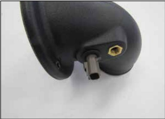
9. Remove the inlet air temperature sensor from the factory housing. Remove the O-Ring from the sensor and then install the sensor into the K&N intake tube using the provided grommet.
