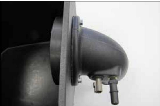
11. Install the bolts and washers into the intake tube, then install the gasket. Now install the tube assembly onto the air box so the bolts pass through the three holes, then install the second gasket and filter adapter. Secure the complete assembly with the provided hardware.
