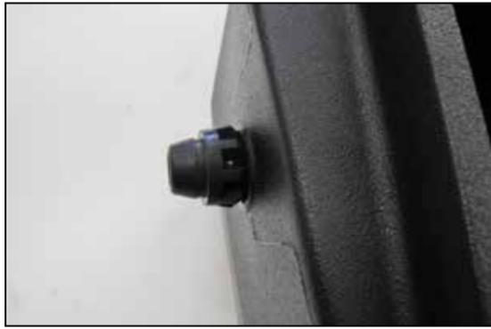
12. Remove the factory air filter housing mounting post and install it onto the K&N air filter housing as shown.
