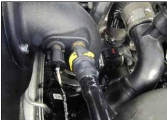
14. Reconnect the inlet air temperature sensor electrical connection and connect the crank case vent line to the fitting installed into the K&N intake tube.
