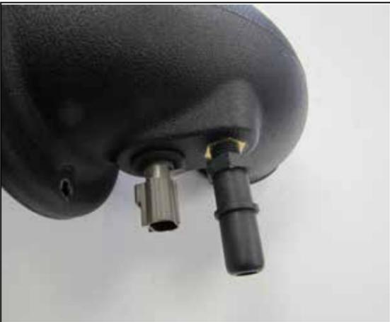
10. Install the provided crank case quick connect fitting into the K&N intake tube as shown.
