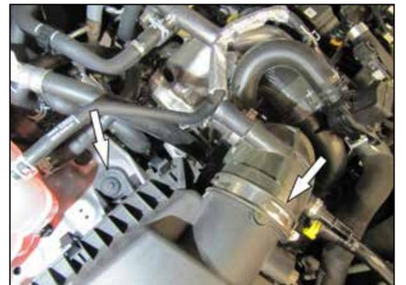
5. Remove the rear air filter housing mounting bolt and loosen the hose clamp that secures the intake hose to the housing.
