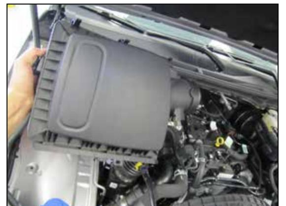
6. Remove the air filter housing from the vehicle.
