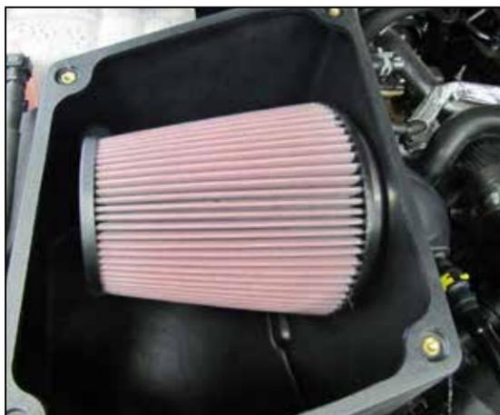
15. Install the K&N air filter onto the filter adapter and secure with the provided hose clamp.
