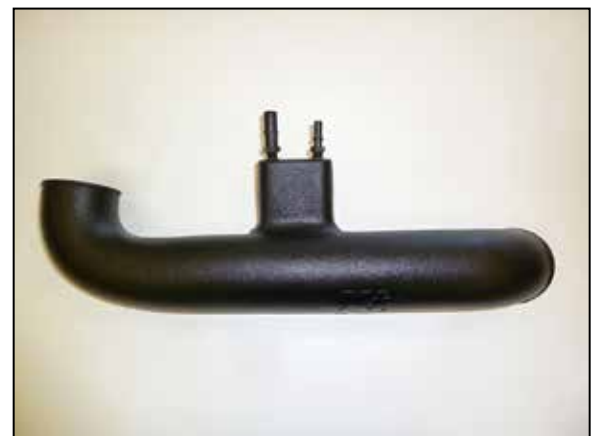
21. Install the provided vent fittings into the K&N® intake tube as shown. NOTE: Plastic NPT fittings are easy to cross thread. Install the vent fitting "hand" tight, then turn it two complete turns with a wrench.
