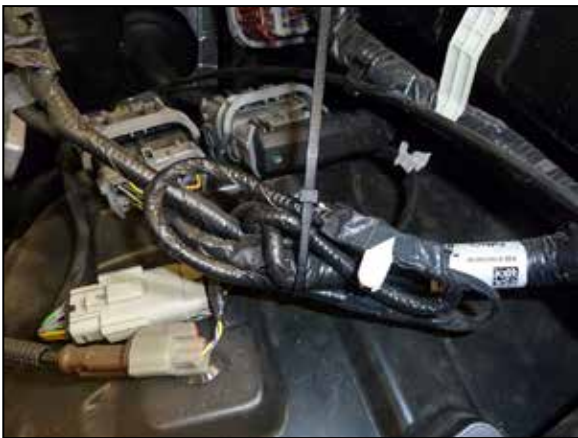
9. On vehicles that have the wiring pig tail that was attached to the lower air filter housing, use the provided tie wrap and secure the pig tail back away from the air filter housing location.
