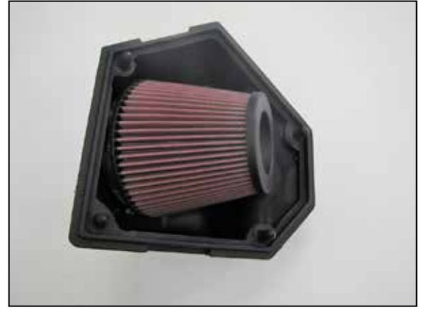
17. Install the filter assembly into the upper K&N® air filter housing and secure with the provided hardware.
