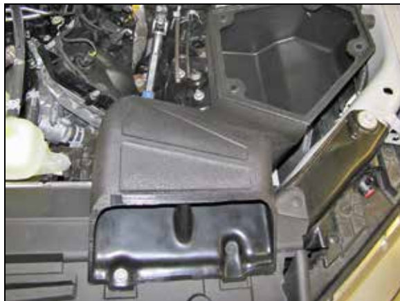
15. Install the two provided retaining clips to secure the fresh air scoop to the core support.
