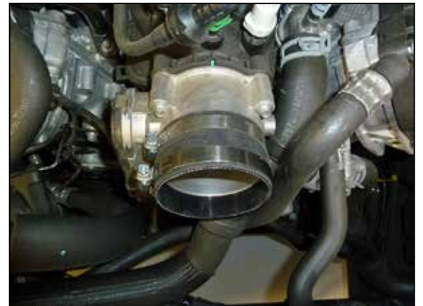
20. Install the provided coupler (08698) onto the throttle body and secure with the provided hose clamp.
