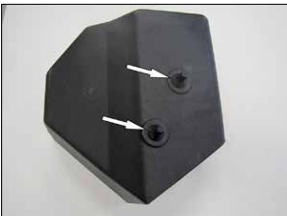
11. Install the two provided mounting studs onto the K&N® filter housing using the provided hardware.
