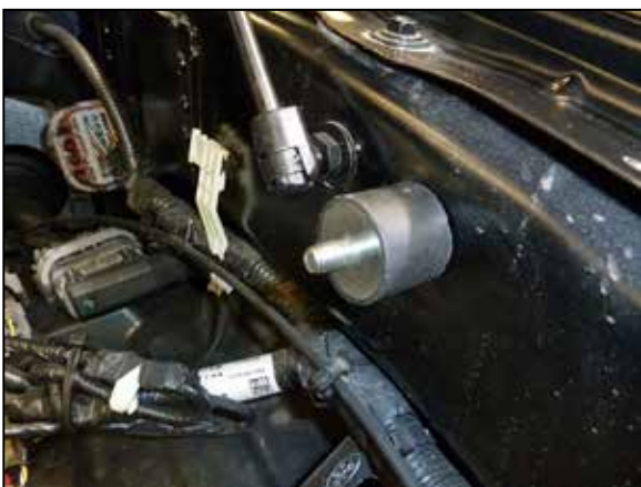
10. Install the provided rubber mounted stud into the factory air filter housing mounting location on the inner fender.
