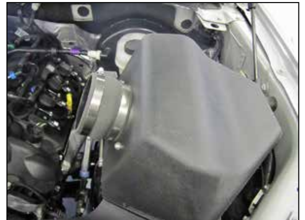
19. Install the provided hump coupler (08639) onto the filter adapter and secure with the provided hose clamp.
