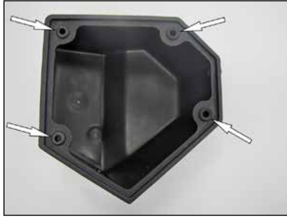
12. Install the four mounting grommets into the K&N® air filter housing as shown.
