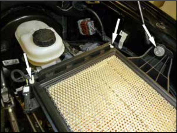
8. On vehicles equipped with the wiring pigtail that secures to the lower air filter housing, disconnect the wiring harness from the lower air filter housing. Remove the bolt that secures the lower air filter housing to the inner fender and then remove the lower housing from the vehicle.
