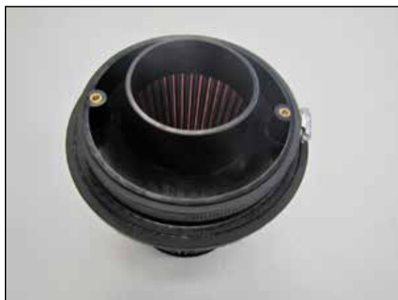
16. Install the K&N® air filter onto the filter adapter and secure with the provided hardware.
