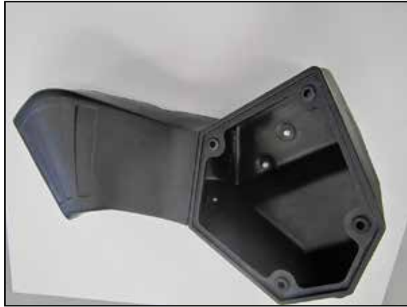
13. Install the K&N® fresh air duct onto the air filter housing and secure with the provided hardware.
