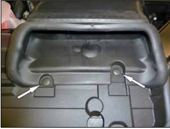
7. Remove the two clips that secure the fresh air intake duct to the core support.
