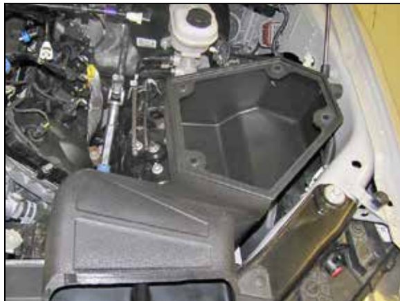
14. Install the K&N® air filter housing assembly into the vehicle and secure to the rubber mounted stud using the provided hardware.
