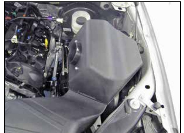
18. Install the upper air filter housing assembly onto the lower filter housing.
