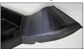
10. Using the provided hardware, secure the K&N® fresh air duct to the lower housing as shown.
