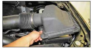
4. Release the two retaining clips that secure the upper air filter housing and then remove the upper housing from the vehicle.
