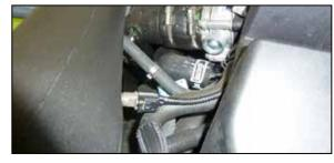
20. Reconnect the inlet air temperature sensor electrical connection using the provided extension harness.
