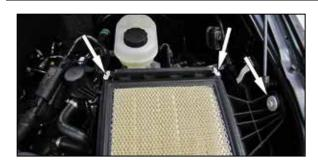
7. Disconnect the wiring harness and purge solenoid from the lower air filter housing if equipped. Remove the bolt that secures the lower air filter housing to the inner fender and then remove the lower housing from the vehicle.
