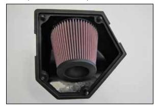
14. Install the air filter assembly into the upper air filter housing and secure with the provided hardware.
