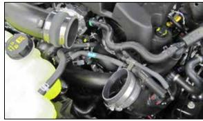
17. Install the provided hump coupler (087121) onto the upper (passenger side) turbo inlet pipe and coupler (08761) onto the lower (Drivers side) turbo inlet pipe and secure with the provided hose clamps.
