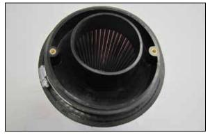
13. Install the filter adapter into the filter and secure with the provided hose clamp.
