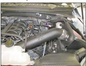
15. Install the K&N® intake into the coupling hose at the filter adapter and then into the hose at the throttle body, adjust the tube for best fit and then secure with the provided hose clamps.
