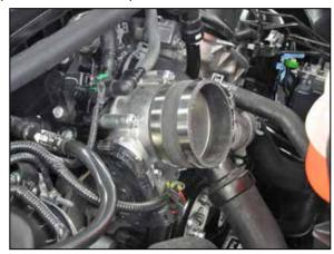
13. Install the provided coupling hose (08698) onto the throttle body and secure with the provided hose clamp.
