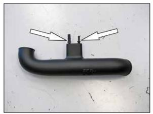
14. Install the two provided quick disconnect fittings into the  $K\&N^{\otimes}$  intake tube as shown.
