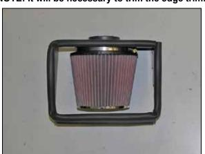
10. <u>Install the air filter onto the filter adapter</u> and secure with the provided hose clamp.
