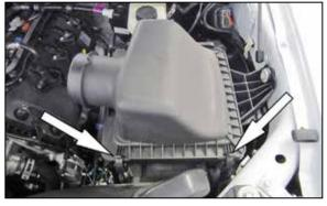
5. Release the two clips securing the upper air filter housing and then remove the upper filter housing and stock air filter.
