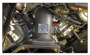
13. Install the tube assembly onto the turbo inlet and into the filter housing. Secure the intake tube with the provided hose clamp and hardware.
