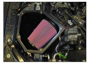
15. Install the K&N<sup>®</sup> air filter onto the intake tube and secure with the provided hose clamp.
