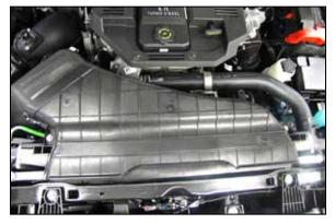
17. Install the K&N<sup>®</sup> fresh air intake duct and then install the factory upper portion of the fresh air intake duct and secure with the factory hardware.
