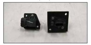
8. Remove the air sensors from the factory housing and install them into the K&N<sup>®</sup> sensor adapters using the provided hardware.
