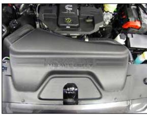
17. Reinstall the factory core support cover and secure with the factory retaining clips.
