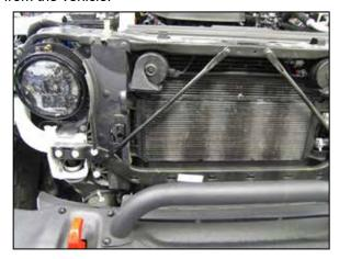
9. Reinstall the core support diagonal brace using the factory hardware.
