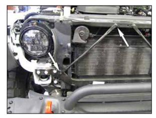
7. Remove the two bolts securing the diagonal core support brace and remove the brace.
