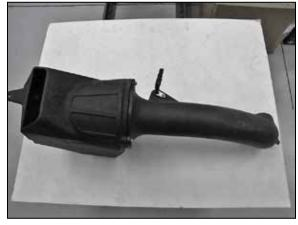
15. Install the intake tube assembly into the K&N<sup>®</sup> air filter housing and secure with the provided hardware.
