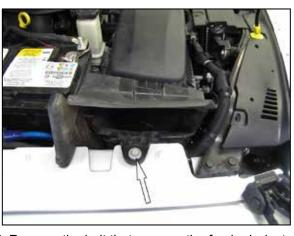
5. Remove the bolt that secures the fresh air duct to the fender. Remove the complete intake system from the vehicle.
