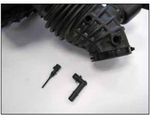
11. Remove the IAT sensor and quick connect CCV fitting from the factory intake tube.
