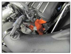
14. Reconnect the CCV quick connect fitting. Reconnect the IAT sensor electrical connection.
