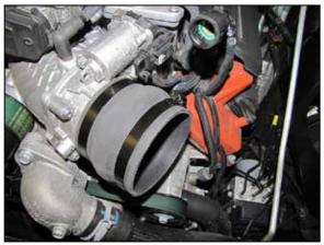
9. Install the provided hump coupler (08418) onto the throttle body and secure with the provided hose clamps.
