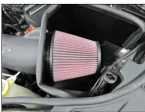
15. Install the K&N® air filter onto the intake tube and secure with the provided hose clamp.
