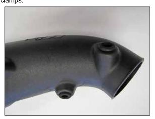
10. Install the provided grommets into the K&N<sup>®</sup> intake tube as shown.
