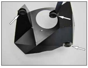
6. Remove the three mounting grommets from the factory air filter housing and install them into the  $K\&N^{\otimes}$  heat shield as shown.
