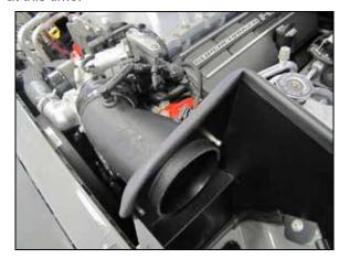
13. Install the K&N® intake tube into the coupling hose and heat shield and secure with the provided hardware to the heat shield.
