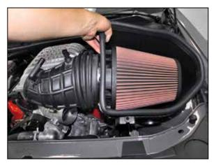
5. Remove the complete factory intake system from the vehicle.
