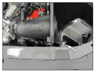
14. Secure the heat shield to the core support with the provided hardware then secure the intake tube with the provided hose clamp.
