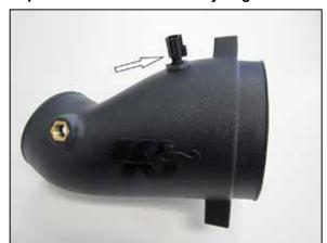
10. Install the provided grommet into the K&N® intake tube, then remove the o-ring from the inlet air temperature sensor and install the sensor into the grommet.
