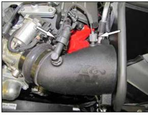
15. Reconnect the inlet air temperature sensor electrical connection and crank case vent line.
