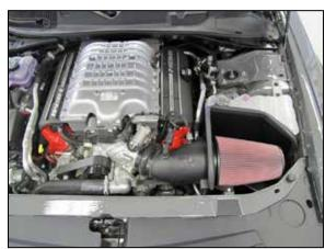
16. Install the K&N® air filter onto the filter adapter and secure with the provided hose clamp.
