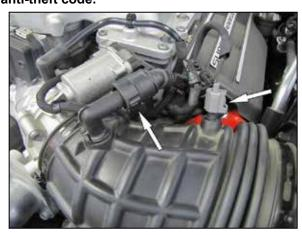
2. Disconnect the inlet air temperature sensor electrical connection and the crank case vent line from the factory intake tube.
