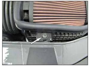
4. Remove the bolt that secures the air filter housing to the core support.
